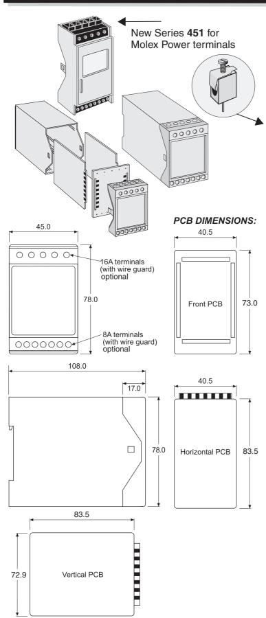
Module enclosure for M36 DIN-rail. To be used in a closed rack or installation box.
