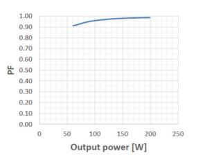
OT 200 2DIM NFC IP67 Typical Power Factor vs. Load
