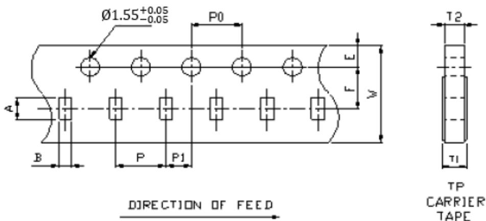
Remark : Pitch tolerance over any 10 pitches of  $P_0$  is  $\pm 0.2$  mm
