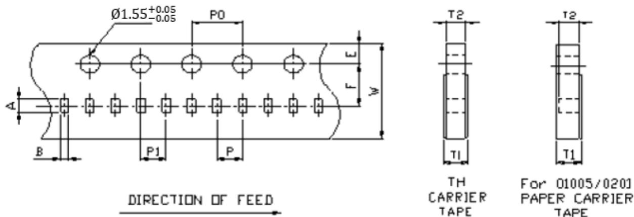
Remark: Pitch tolerance over any 10 pitches of P<sub>0</sub> is  $\pm 0.2$  mm
