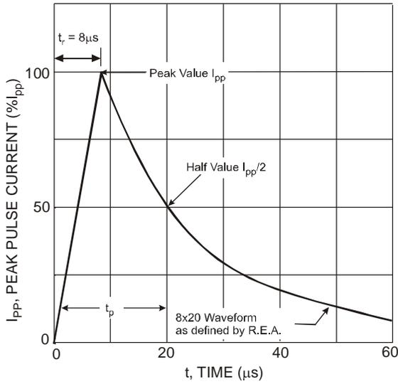
Figure 3 Typical 8 × 20µs Pulse Waveform
