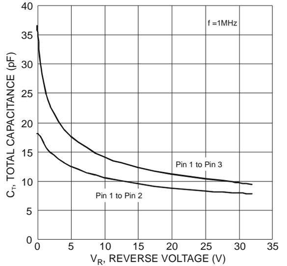
Figure 4 Typical Total Capacitance vs. Reverse Voltage
