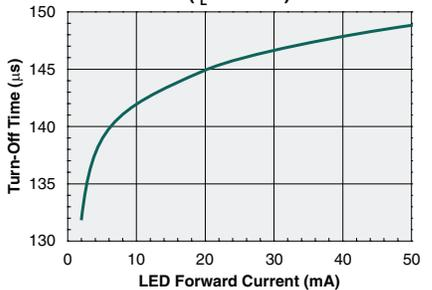
**Typical  $I_F$  for Switch Operation**
