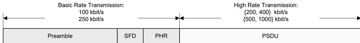
Due to the overhead caused by the PPDU header and the FCS, the effective data rate is less than the selected data rate, depending on the length of the PSDU.
