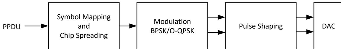
The combination of spreading, modulation and pulse shaping are restricted to several combinations, as shown in the following table.
