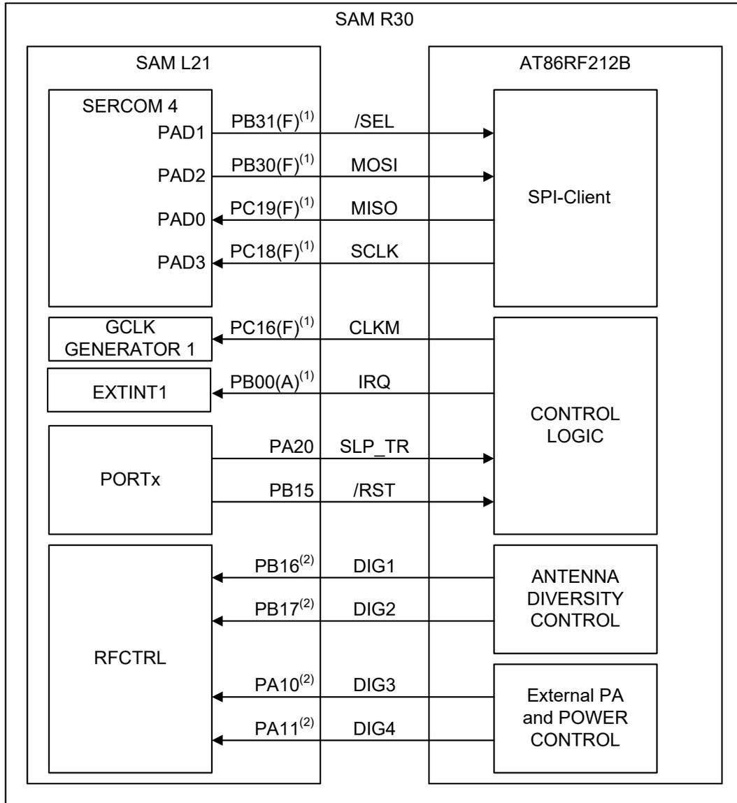
1. Alternate pin function and direction has to be configured by software.
