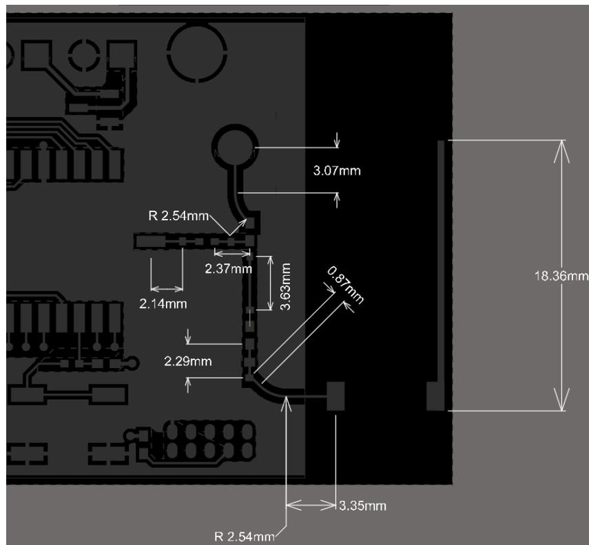
Figure 12-5. Layer 2 (GND) Layout
