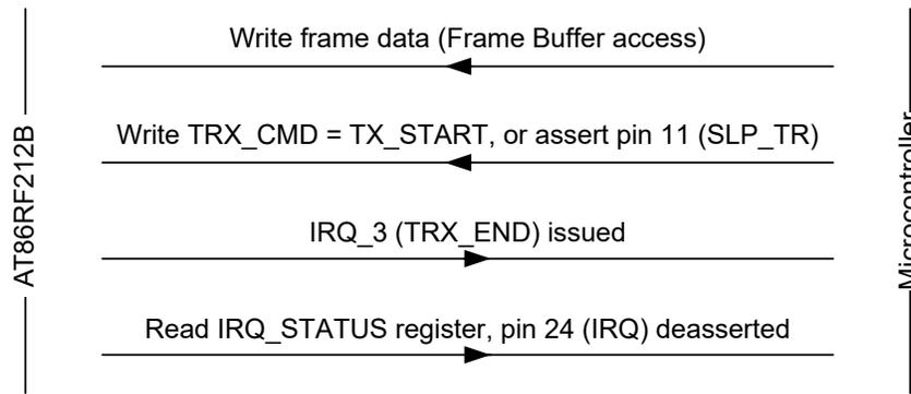
Alternatively, for time critical applications when the frame start transmission time needs to be minimized, a frame transmission task can be started first. Then it can be followed by the Frame Buffer write access event (populating PSDU data). This way the data to be transmitted needs to be written in the transmit frame buffer as the transceiver initializes and begins the SHR transmission.
