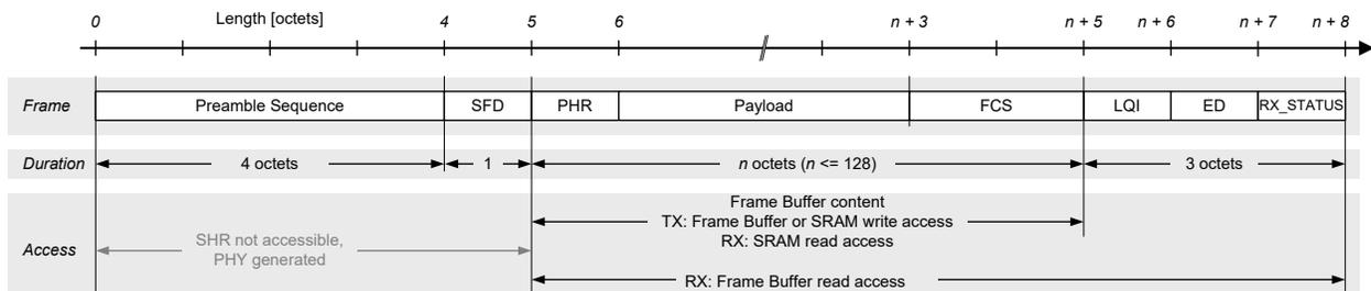
A frame comprises two sections, the radio transceiver internally generated SHR field and the user accessible part stored in the Frame Buffer. The SHR contains the preamble and the SFD field. The variable frame section contains the PHR and the PSDU including the FCS.
