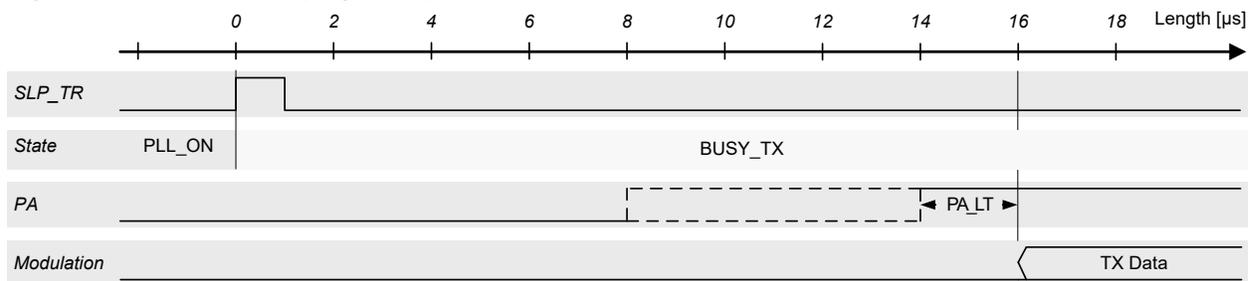
Using an external RF front-end, it may be required to adjust the start-up time of the external PA relative to the internal building blocks to optimize the overall PSD. This can be achieved using the RF\_CTRL\_0.PA\_LT bits.
