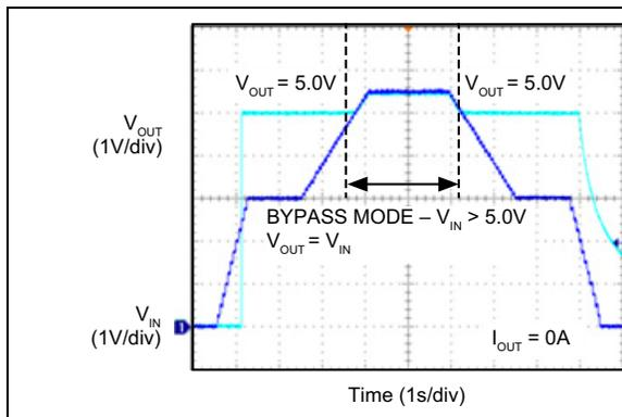
**FIGURE 2-20:** Bypass Mode.
