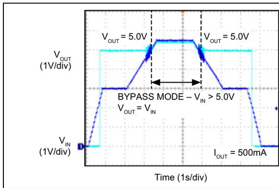
**FIGURE 2-21:** Bypass Mode.
