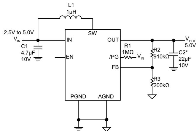
\*Two more 22 µF capacitors should be added in parallel with C2 for  $V_{IN} > 5.0V$ .
