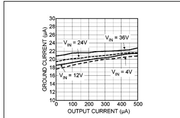
**FIGURE 2-6:** Ground Pin Current vs. Output Current.
