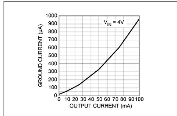
**FIGURE 2-5:** Ground Pin Current vs. Output Current.
