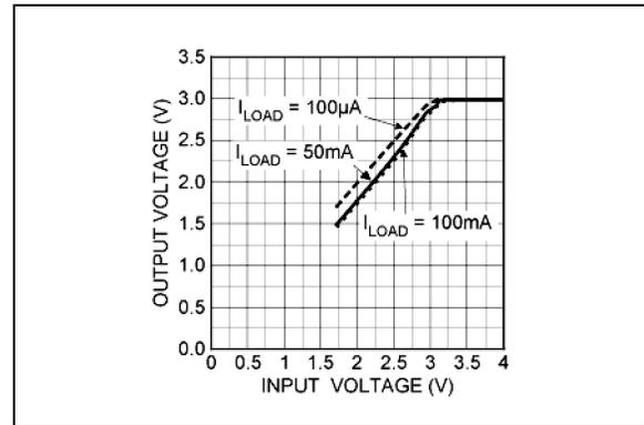
**FIGURE 2-4:** Dropout Characteristics.
