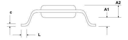
28-Pin SSOP Package Dimensions
