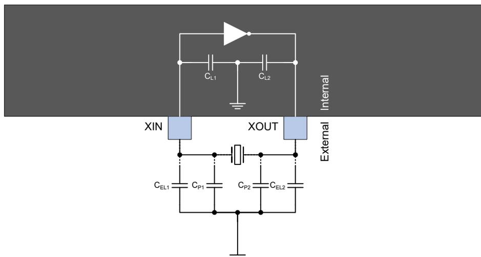
Using this model the total capacitive load for the crystal can be calculated as shown in the equation below:
