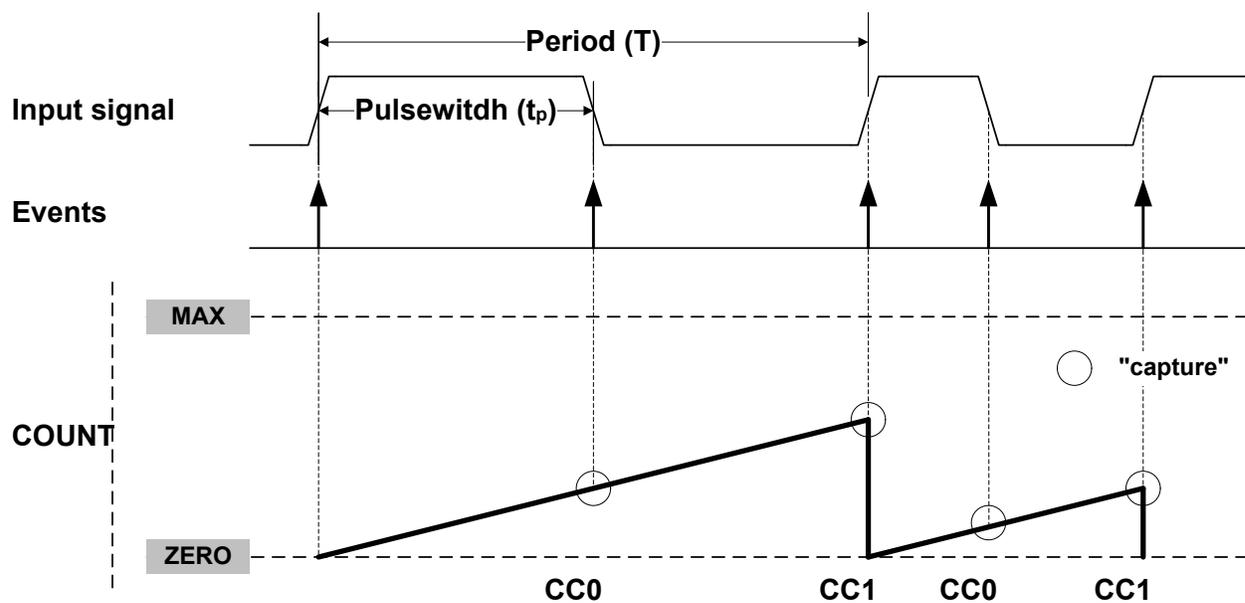
Selecting PWP in the Event Action bit group in the Event Control register (EVCTRL.EVACT) enables the TC to perform one capture action on the rising edge and another one on the falling edge. The
