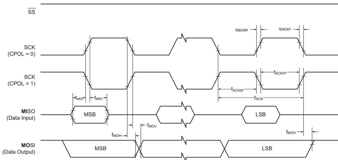
Figure 48-3. SPI Timing Requirements in Client Mode
