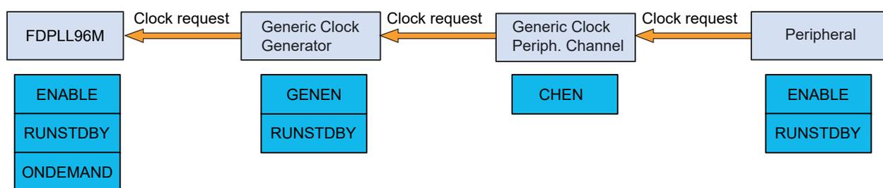
All clock sources in the system can be run in an on-demand mode: the clock source is in a stopped state unless a peripheral is requesting the clock source. Clock requests propagate from the peripheral, through the GCLK, to the clock source. If one or more peripheral is using a clock source, the clock source will be started/kept running. As soon as the clock source is no longer needed and no peripheral has an active request, the clock source will be stopped until requested again.
