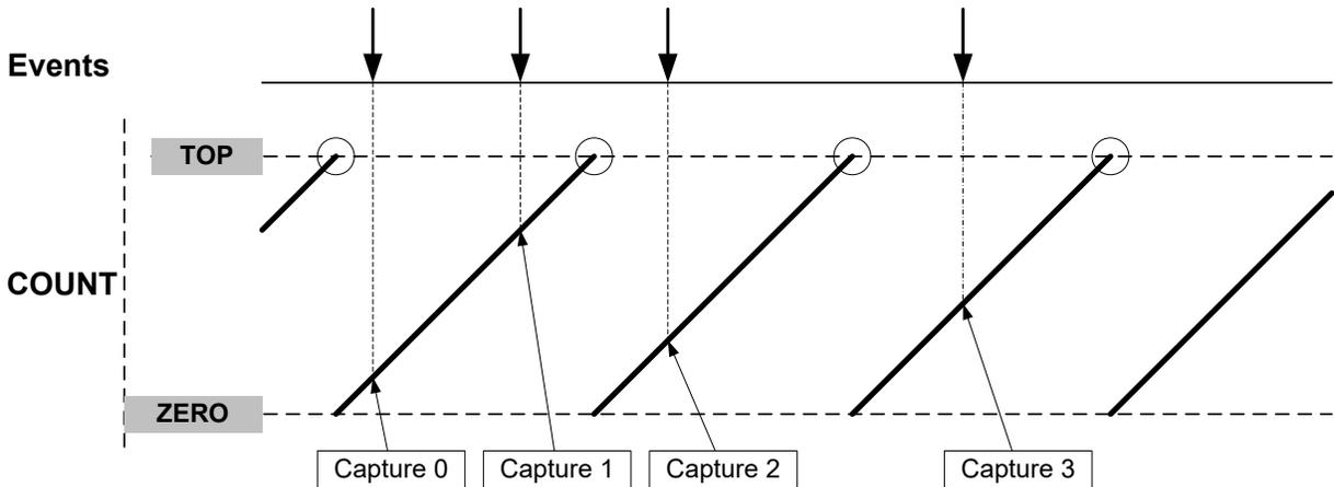
The TC can detect capture overflow of the input capture channels: When a new capture event is detected while the Capture Interrupt flag (INTFLAG.MCx) is still set, the new timestamp will not be stored and INTFLAG.ERR will be set.
