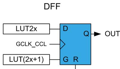
When the even LUT is disabled (LUTCTRL(2n).ENABLE=0), the flip-flop is asynchronously cleared. The reset command (R) is kept enabled for one APB clock cycle. In all other cases, the flip-flop output (OUT) is refreshed on rising edge of the GCLK\_CCL, as shown in [Table 40-2](#).
