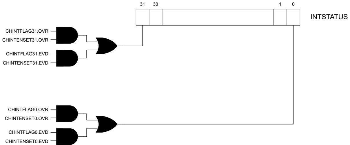
The Event System can arbitrate between all channels with pending interrupts. The arbiter can be configured to prioritize statically or dynamically the incoming events. The priority is evaluated each time a new channel has an interrupt pending, or an interrupt has been cleared. The Channel Pending Interrupt register (INTPEND) will provide the channel number with the highest interrupt priority, and the corresponding channel interrupt flags and status bits.
