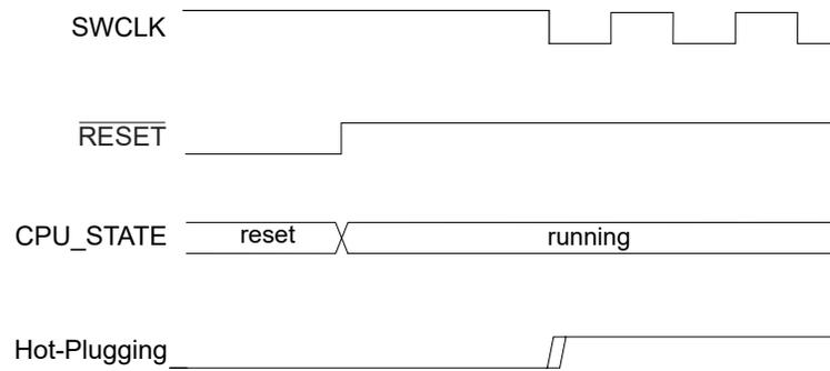
The presence of a debugger probe is detected when either Hot-Plugging or Cold-Plugging is detected. Once detected, the Debugger Present bit of the Status B register (STATUSB.DBGPRES) is set. For security reasons, Hot-Plugging is not available when DAL equals to 0x0.
