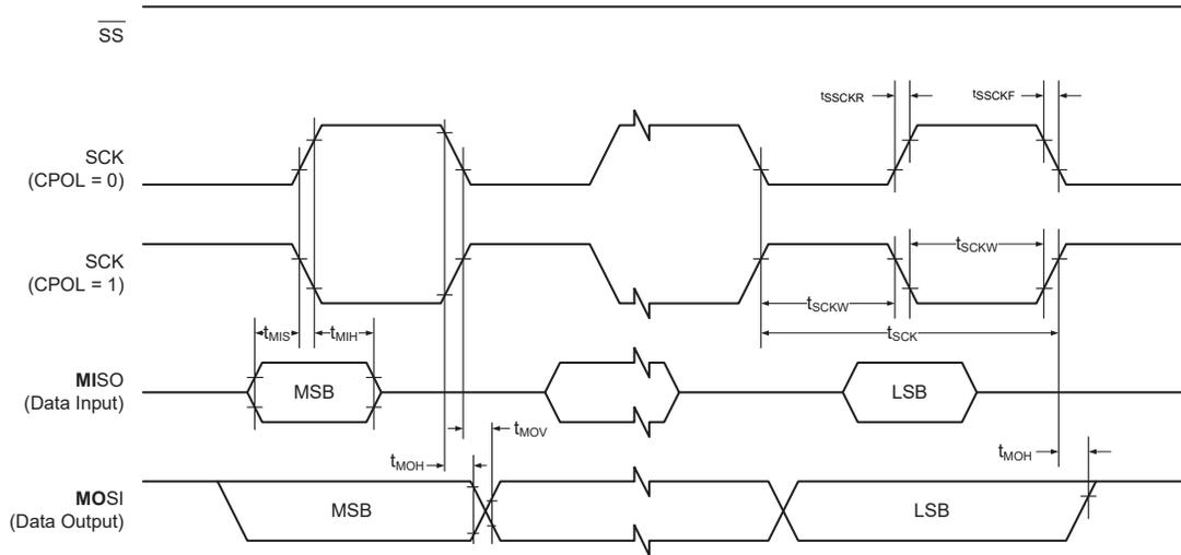
**Figure 48-5. SPI Timing Requirements in Client Mode**
