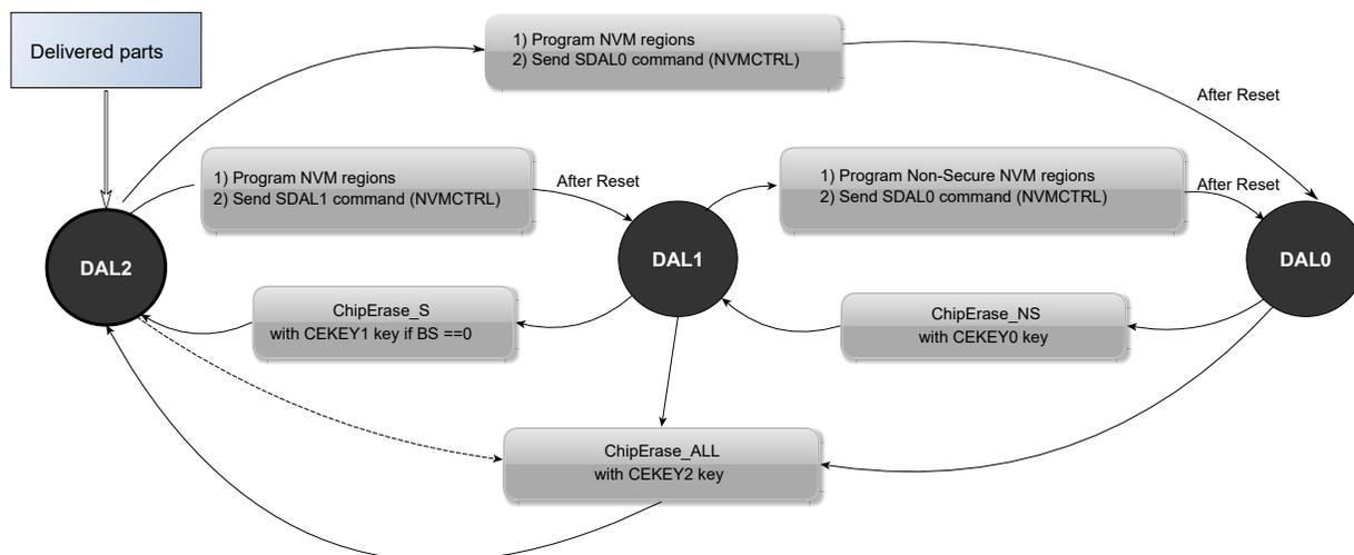
Decreasing the Debug Level Access is done using the NVMCTRL peripheral command from the debugger or the CPU.
