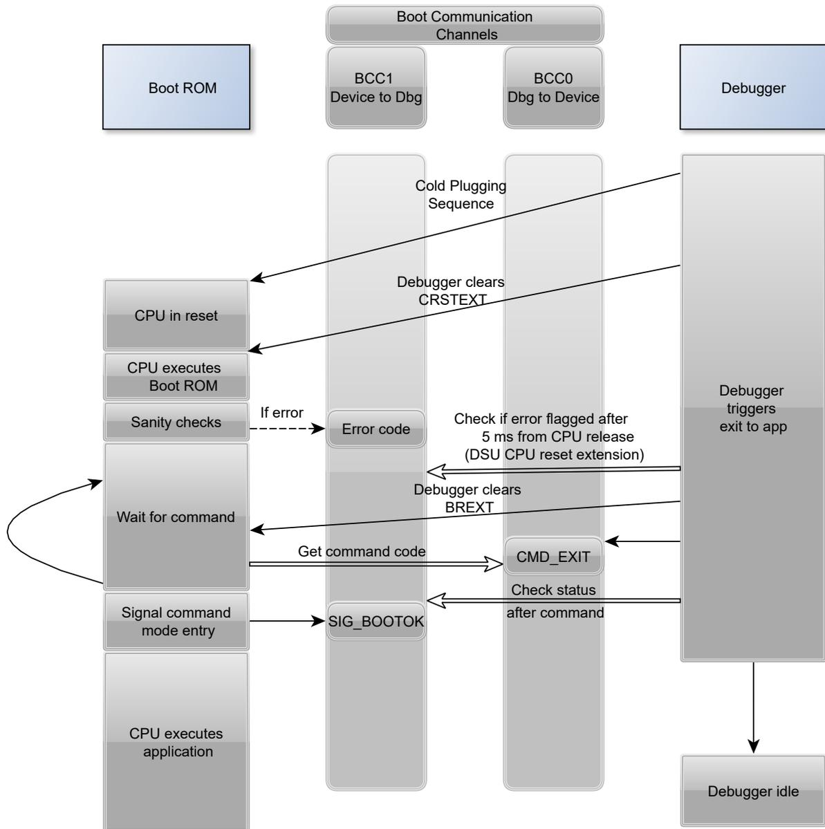
Figure 14-9. CMD\_EXIT to Park mode flow diagram
