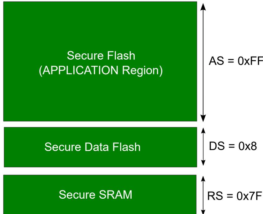
Here is a typical configuration for a device with 64KB of Flash, 2KB of Data Flash and 16KB of SRAM:
