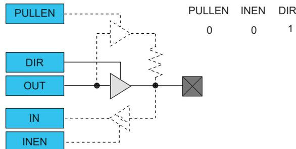
Figure 32-7. I/O Configuration - Totem-Pole Output with Enabled Input
