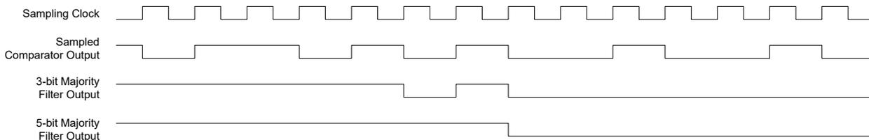
**Figure 42-7. Single-Shot Filtering**
