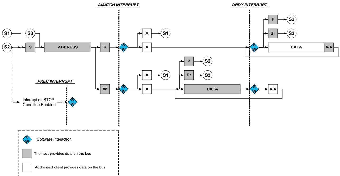
In the second strategy (CTRLA.SCLSM=1), interrupts only occur after the ACK bit is sent as shown in the following figure. This strategy can be used when it is not necessary to check DATA before acknowledging. For host reads, an address and data interrupt will be issued simultaneously after the address acknowledge. However, for host writes, the first data interrupt will be seen after the first data byte has been received by the client and the acknowledge bit has been sent to the host.
