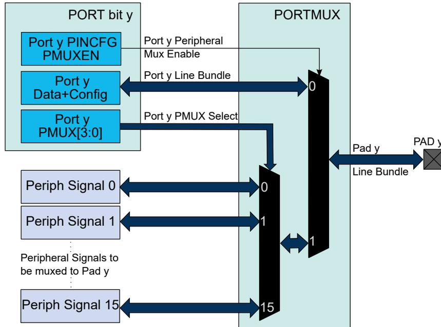
The I/O pins of the device are controlled by PORT peripheral registers. Each port pin has a corresponding bit in the Data Direction (DIR) and Data Output Value (OUT) registers to enable that pin as an output and to define the output state.
