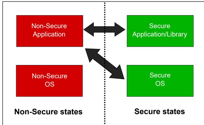
If the TrustZone is implemented (SAM L11 devices), the system starts up in Secure state by default. The security state of the processor can be either Secure or Non-Secure.
