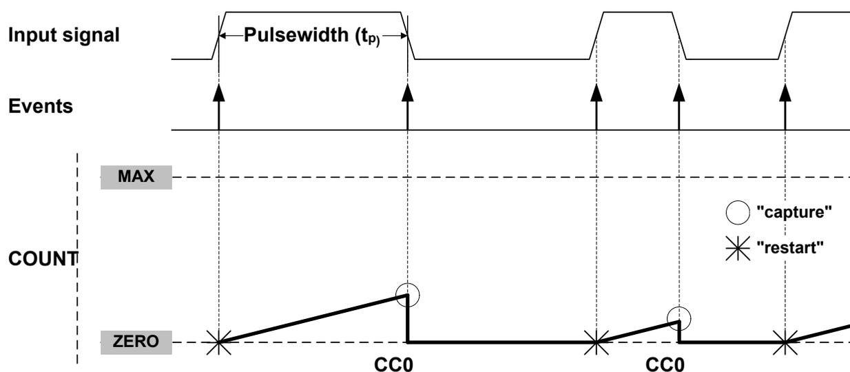
The TC can detect capture overflow of the input capture channels: When a new capture event is detected while the Capture Interrupt flag (INTFLAG.MCx) is still set, the new timestamp will not be stored and INTFLAG.ERR will be set.
