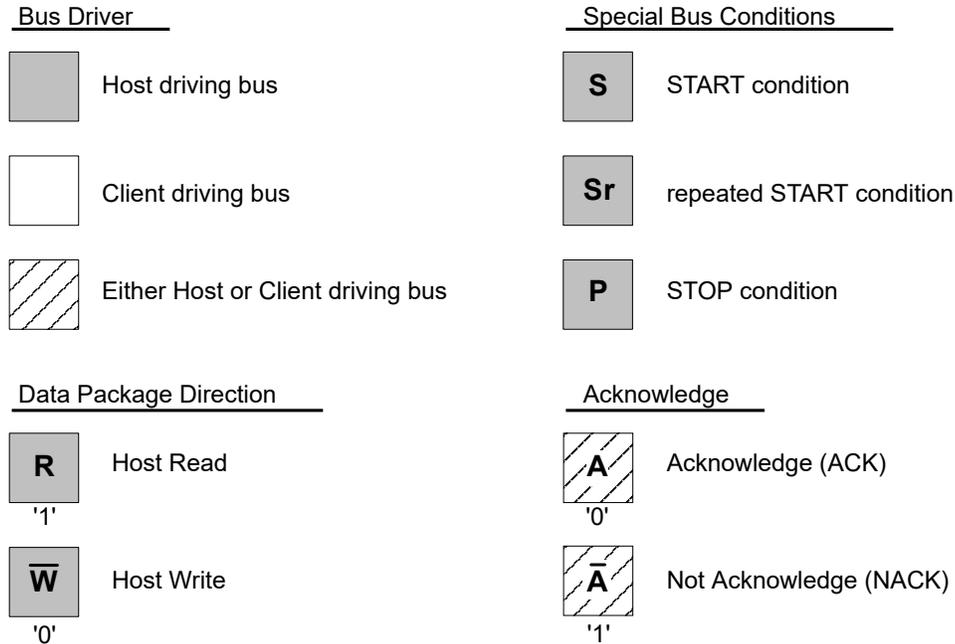
Figure 37-3. Basic I<sup>2</sup>C Transaction Diagram
