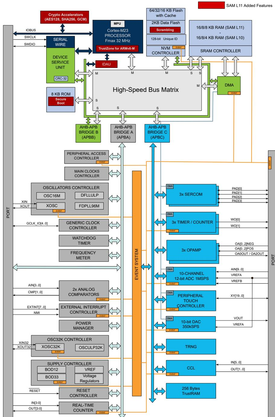
**Note:** Number of SERCOM instances, PTC/ADC channels, Tamper input pins, and Analog Compare inputs differ on the packages pinout.
