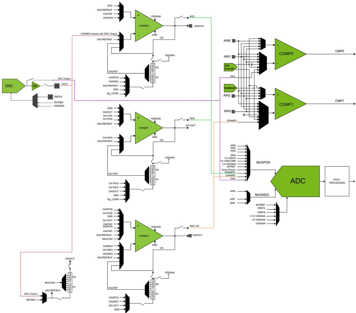
**Note:** Some OPAMP Outputs (OA<sub>x</sub>OUT) can be connected directly to specific Analog Comparator or ADC Inputs (AIN<sub>x</sub>) if they share the same pad, for example, OA0OUT can be connected to the Analog Comparator AIN3 or ADC AIN5 input (PA07 pin).
