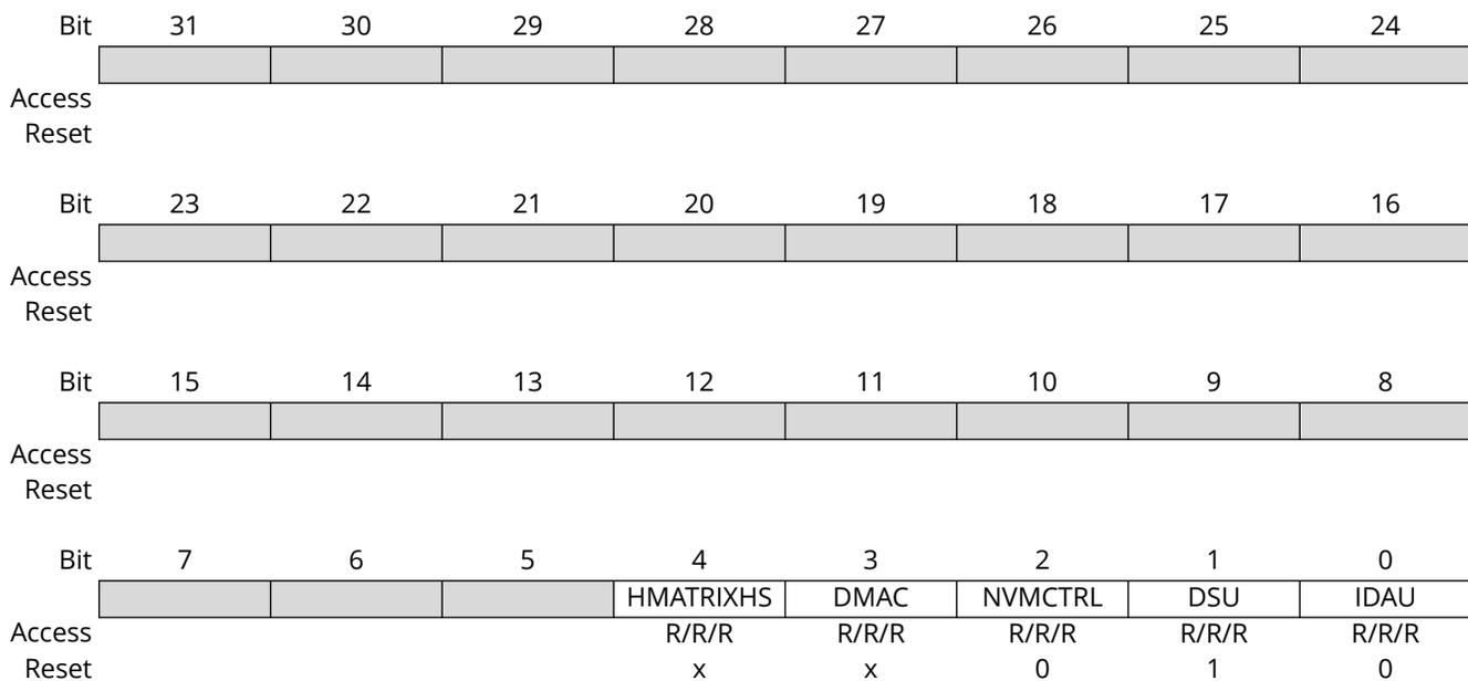
**Bit 4 - HMATRIXHS** Peripheral HMATRIXHS Non-Secure
