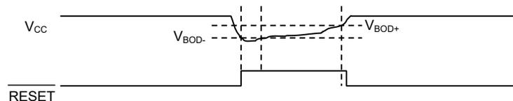
Enabling the BOD33 hysteresis by writing the Hysteresis bit in the BOD33 register (BOD33.HYST) to '1' will add hysteresis to the BOD33 threshold level.
