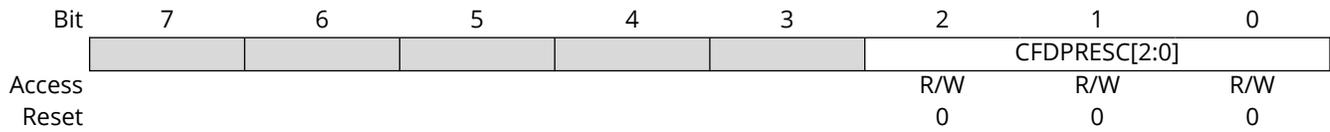
**Bits 2:0 – CFDPRESC[2:0]** Clock Failure Detector Prescaler
