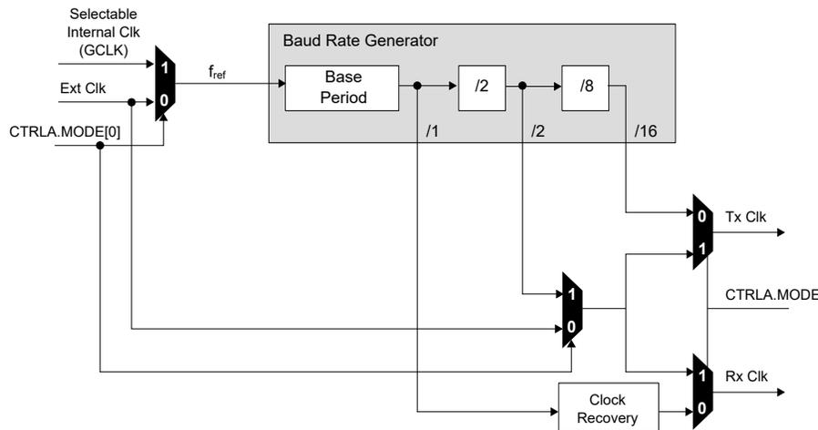
Table 34-3 contains equations for the baud rate (in bits per second) and the BAUD register value for each operating mode.
