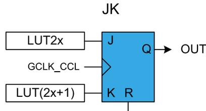
When the even LUT is disabled (LUTCTRL(2n).ENABLE=0), the flip-flop is asynchronously cleared. The reset command (R) is kept enabled for one APB clock cycle. In all other cases, the flip-flop output (OUT) is refreshed on rising edge of the GCLK\_CCL, as shown in the following table.
