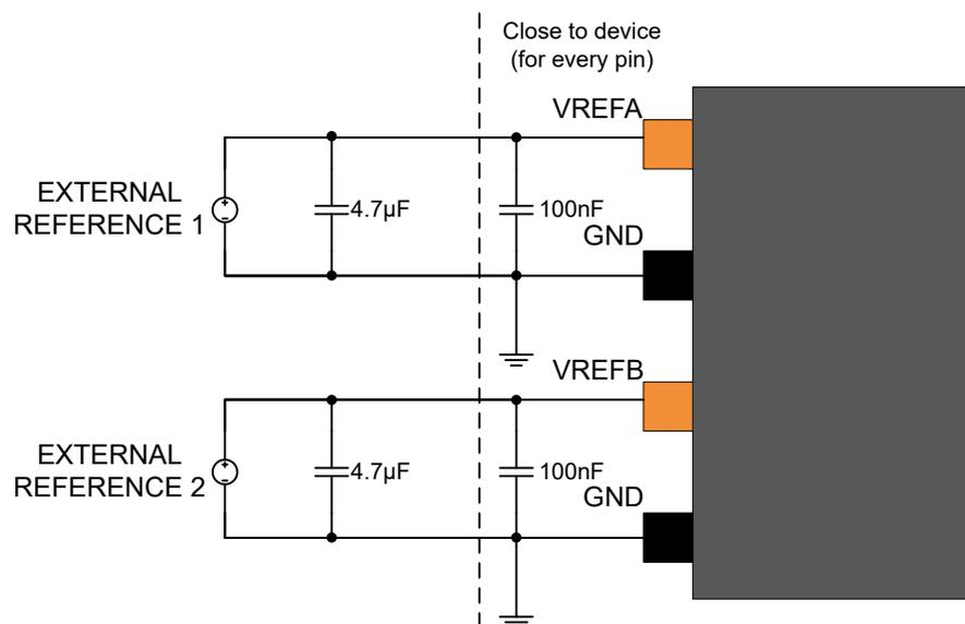
Figure 51-4. External Analog Reference Schematic With One Reference
