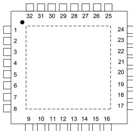
Figure 4-4. SAM L10/L11 32-pin WLCSP Pinout
