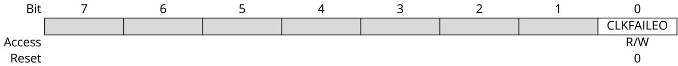
**Bit 0 – CLKFALEO** Clock Failure Detector Event Out Enable
