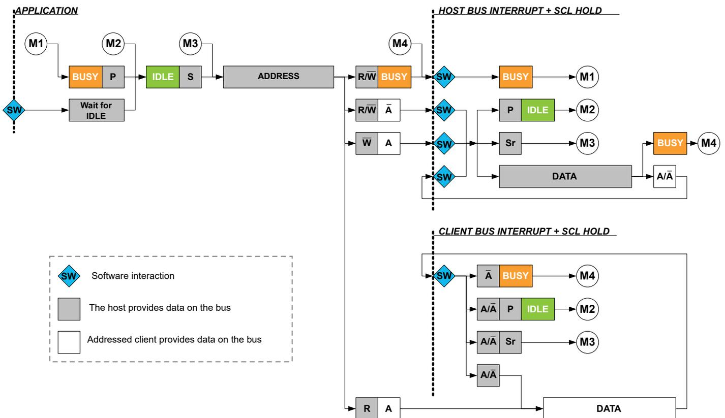
In the second strategy (CTRLA.SCLSM=1), interrupts only occur after the ACK bit, as shown in the following figure. This strategy can be used when it is not necessary to check DATA before acknowledging.
