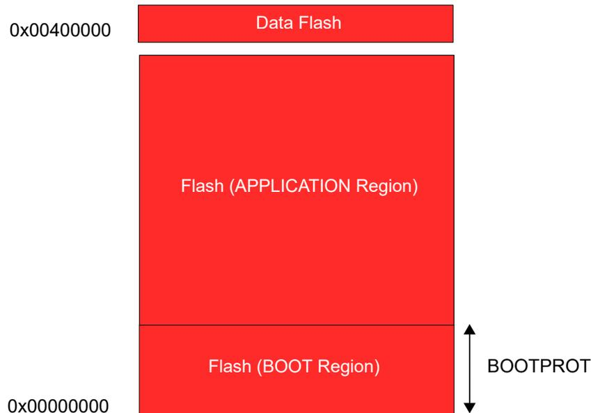
The lower rows in the FLASH can be allocated as a boot loader section by using the BOOTPROT fuses.
