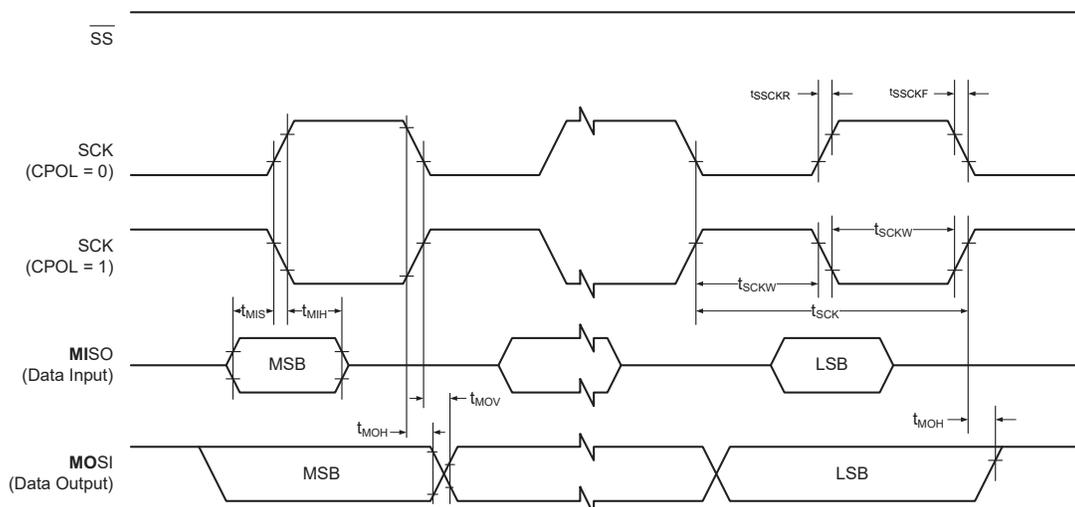
Figure 46-6. SPI Timing Requirements in Client Mode
