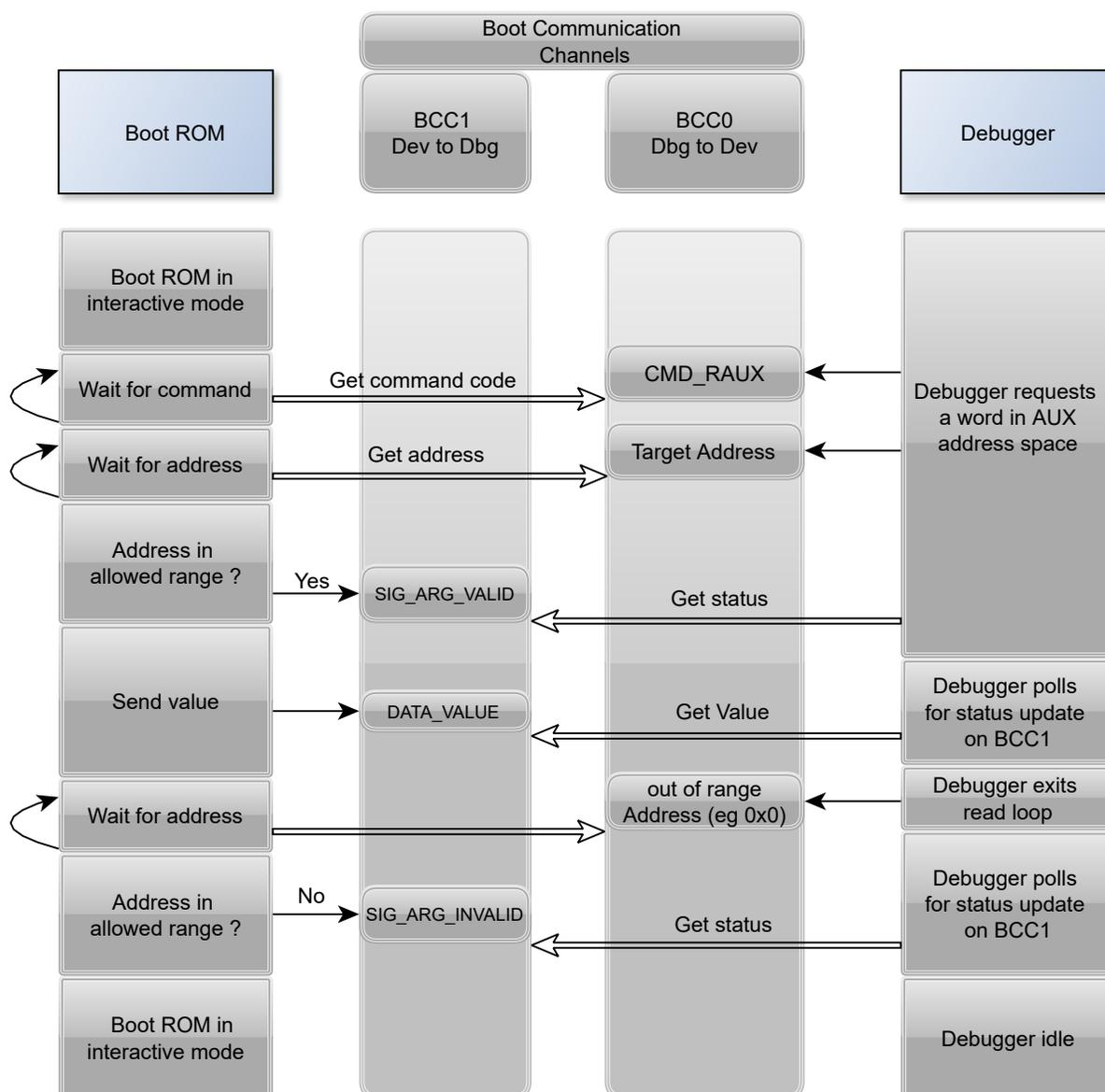
Note: After the CMD\_RAUX is sent, the debugger can read multiple data, the read loop is exit when an out of range address is sent.
