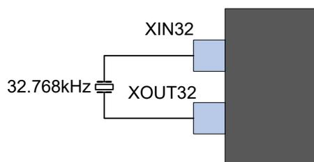
To improve accuracy and safety, it is recommended to add external capacitors, as recommended in the crystal data sheet. See figure below for additional information.
