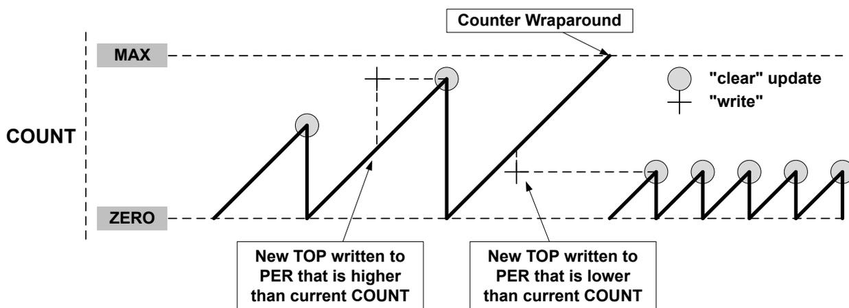
A counter wraparound can occur in any operation mode when up-counting without buffering, refer to the following figure.
