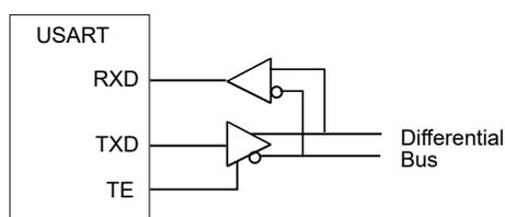
The TE pin will remain high for the complete frame including stop bit(s). If a Guard Time is programmed in the Control C register (CTRLC.GTIME), the line will remain driven after the last character completion. The following figure shows a transfer with one stop bit and CTRLC.GTIME=3.
