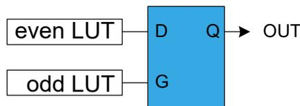
When the even LUT is disabled (LUTCTRL(2n).ENABLE=0), the latch output will be cleared. The G-input is forced enabled for one more APB clock cycle, and the D-input to zero. In all other cases, the latch output (OUT) is refreshed as shown in the following table.
