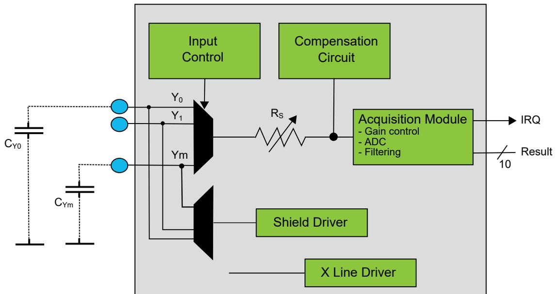
**Note:** For SAM L10/L11 the  $R_S = 100\text{ K}\Omega$ .
