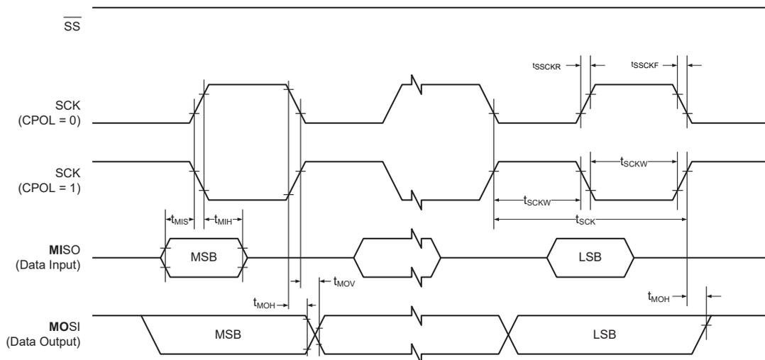
**Figure 47-3. SPI Timing Requirements in Client Mode**
