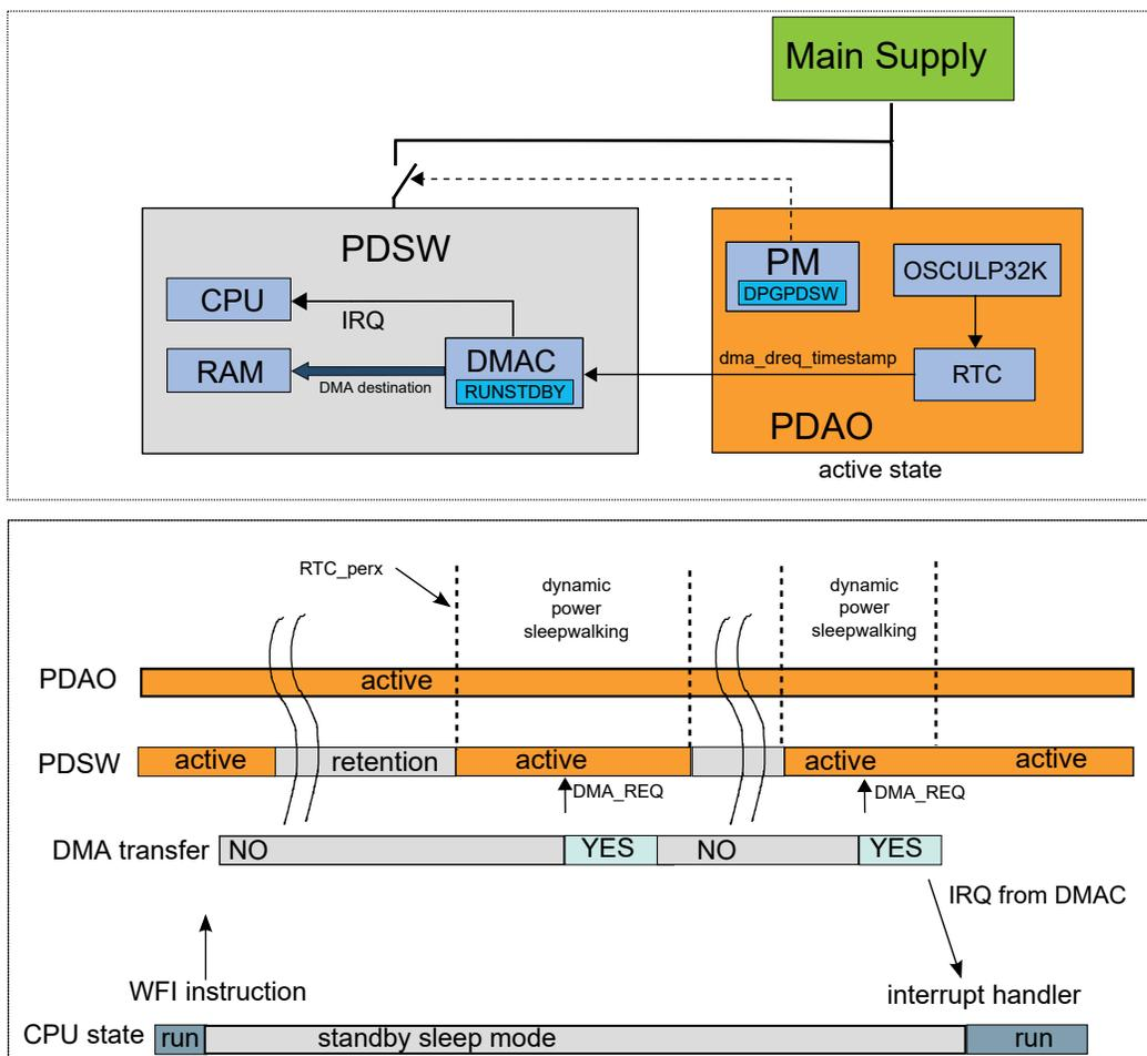
The DMAC is configured to operate in standby sleep mode by using its respective RUNSTDBY bit. A DMAC channel is configured to set the DMA destination. The Run in Standby bit of this DMAC channel is written to '1' to allow it running in Standby Sleep mode.
