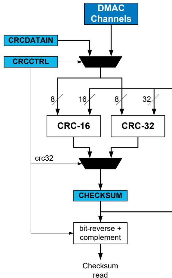
**CRC on DMA data** CRC-16 or CRC-32 calculations can be performed on data passing through any DMA channel. Once a DMA channel is selected as the source, the CRC engine will continuously generate the CRC on the data passing through the DMA channel. The checksum is available for readout once the DMA transaction is completed or aborted. A CRC can also
