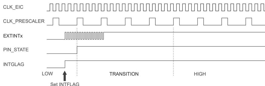
In this mode, the EIC clock is requested. The asynchronous edge detection mode can be used in Idle and Standby sleep modes.
