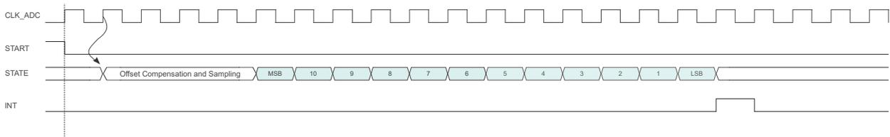
The following figure shows the ADC timing for free-running mode conversion.
