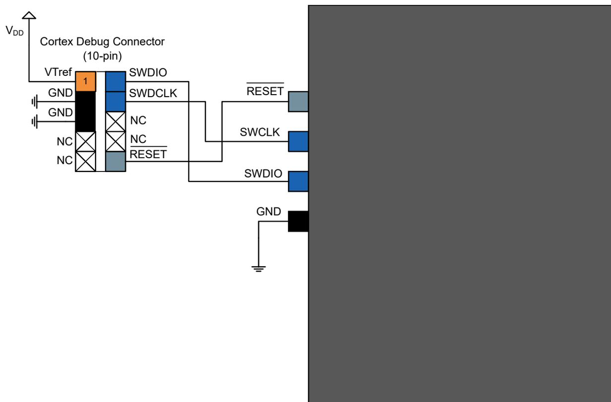
**Table 51-7.** Cortex Debug Connector (10-pin)
