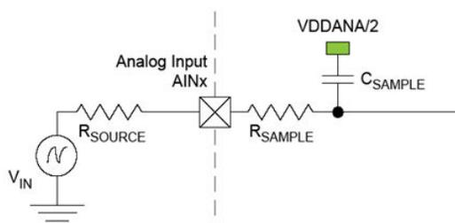
The minimum sampling time  $t_{\text{samplehold}}$  for a given  $R_{\text{source}}$  can be calculated using the following formula:
