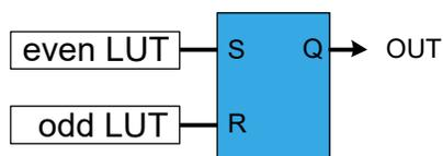
When the even LUT is disabled (LUTCTRL(2n).ENABLE=0), the latch output will be cleared. The R-input is forced enabled for one more APB clock cycle and S-input to zero. In all other cases, the latch output (OUT) is refreshed as shown in the following table.
