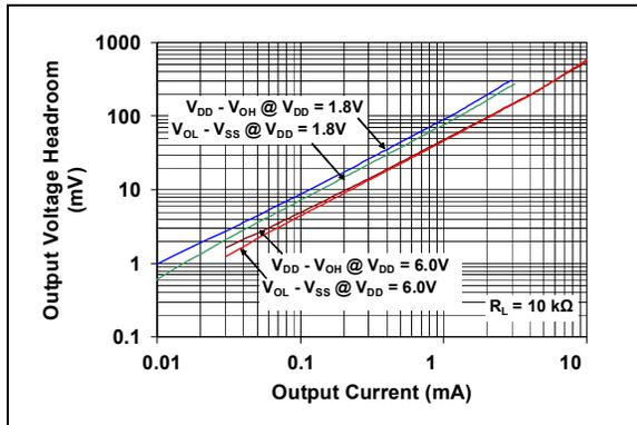
**FIGURE 2-26:** Output Voltage Headroom vs. Output Current.
