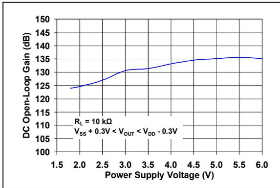
**FIGURE 2-20:** DC Open-Loop Gain vs. Power Supply Voltage.
