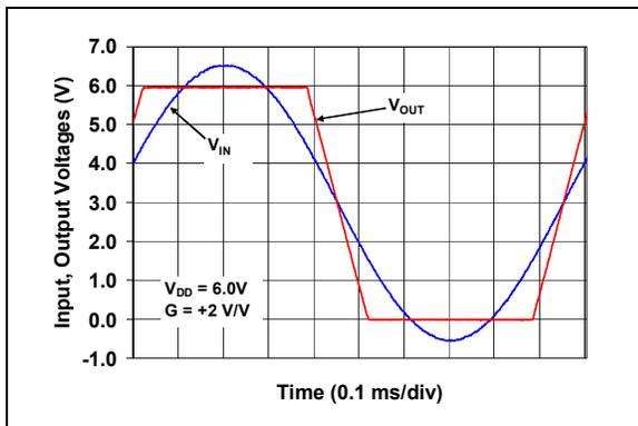
**FIGURE 2-33:** The MCP6401/1R/1U/2/4/6/7/9 Shows No Phase Reversal.
