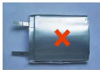
Cell extrusion distortion
