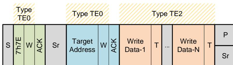
**Figure 37-58.** Private Write Transfer Initiated with Restart Condition (w/ 7'h7E) Error Type Frame Format
