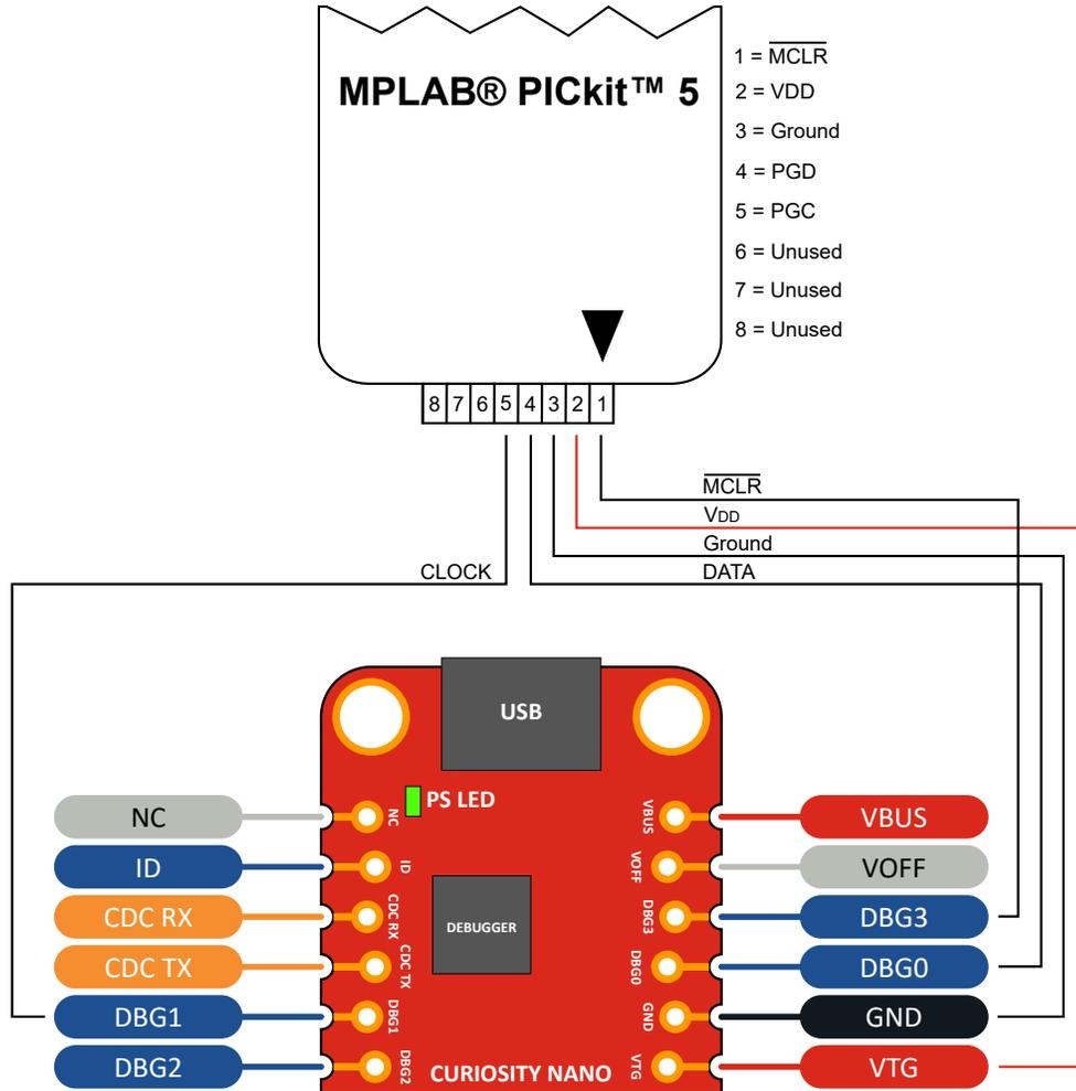
**CAUTION** The MPLAB® PICKit™ 5 In-circuit Debugger/Programmer can deliver high voltage on the  $\overline{\text{MCLR}}$  pin. High voltage can permanently damage R209. If R209 is broken, the on-board debugger cannot enter the programming mode of the PIC18F16Q20 and will typically fail at reading the device ID.
