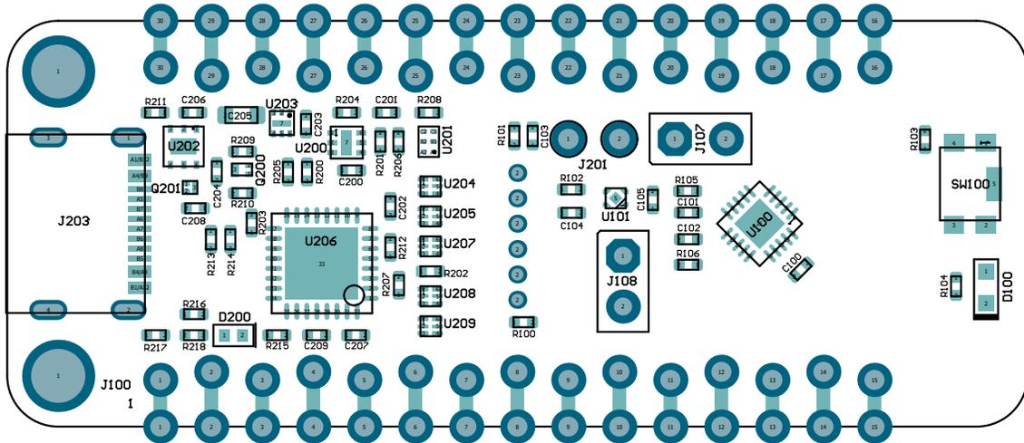
Figure 6-4. PIC18F16Q20 Curiosity Nano Assembly Drawing Bottom
