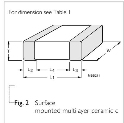
Fig. 2 Surface mounted multilayer ceramic c
