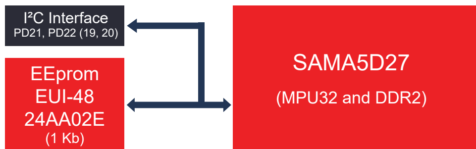
Figure 5-5. EEPROM Memory Block Diagram
