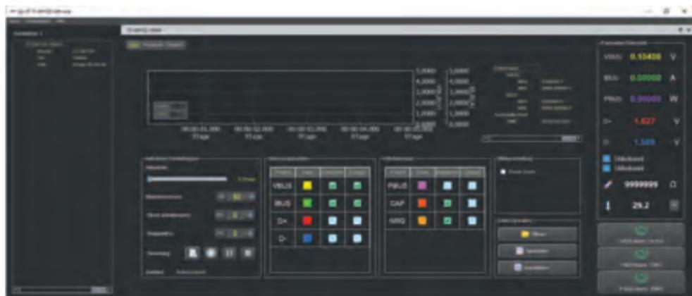
**RECORDING:** The voltage (VBUS), current (IBUS), power (PBUS), data signals (D+ and D-), and capacitance (CAP) and energy (NRG) can be recorded, and the recording conditions such as start and stop current and sampling rate can be configured.
