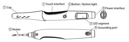
①Touch interface: Press/touch enables the machine heating. Together with the ② button, it allows temp. calibration, temp. setting, and other functions.
