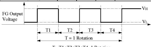
T=T1+T2+T3+T4=1 Rotation  $T=\frac{60}{\text{rpm}}$
