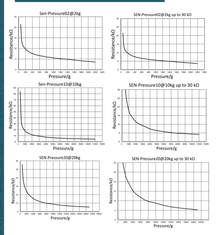
The diagram on the left shows the pressure-resistance relationship for the entire resistance range. The right diagram is a partial section of the left diagram and shows the pressure-resistance relationship normalized for resistance values up to  $30 \text{ k}\Omega$ .
