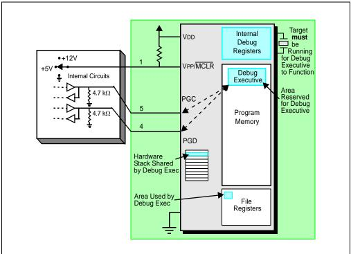
Typically, to find out whether an application program will run correctly, a breakpoint is set early in the program code. When a breakpoint is set from the user interface of MPLAB X IDE, the address of the breakpoint is stored in the special internal debug registers of the target device. Commands on PGC and PGD communicate directly to these registers to set the breakpoint address.
