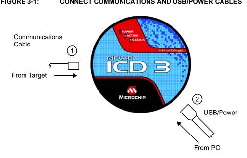
FIGURE 3-1: CONNECT COMMUNICATIONS AND USB/POWER CABLES
