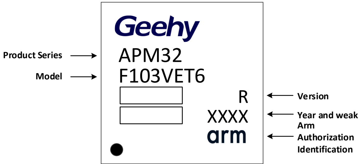
Figure 22 LQFP100 - 100 pin, 14 x 14mm package identification diagram
