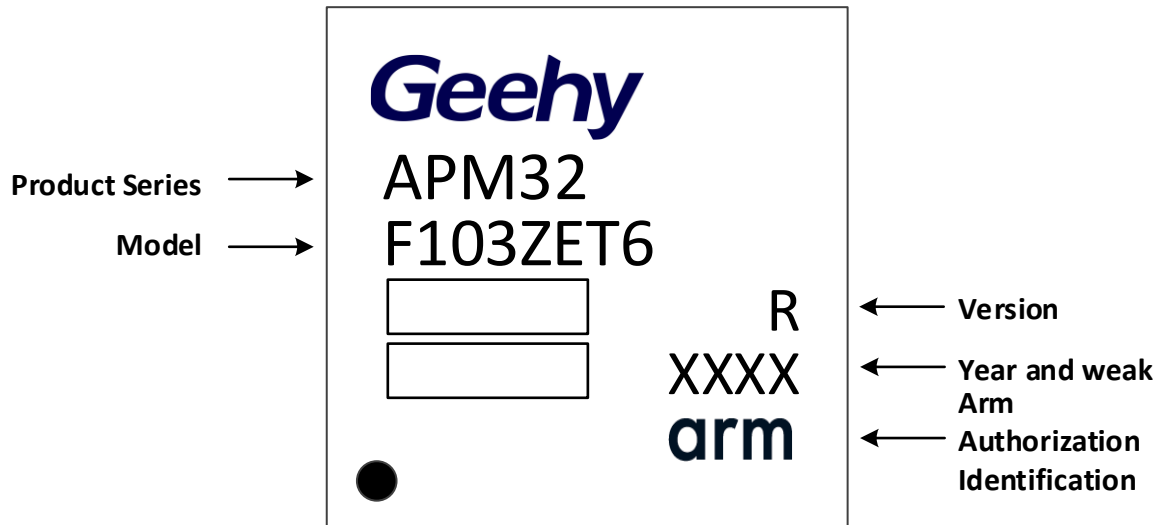
Figure 19 LQFP144-144 pin, 20 x20 mm package identification diagram
