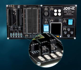
**UART (Universal Asynchronous Receiver/Transmitter):** This interface enables asynchronous serial communication via two lines: TX (Transmit) and RX (Receive). UART is often used for communication between microcontrollers and computers or for connecting modules such as GPS receivers or Bluetooth modules.
