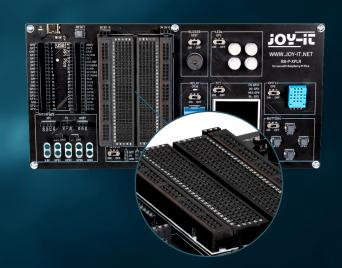
**The main areas:** These consist of a series of parallel rows of holes, usually separated by a central groove. The holes within a row are electrically connected to each other. This arrangement is ideal for inserting integrated circuits (ICs) and other components.
