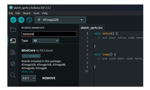
Now select the appropriate board: **Tools** → **Board** → **Minicore** → **ATmega328** At **Tools** → **Port**, select the port to which your device is connected. At **Tools** → **Variant**, select **328PB**. And at **Tools** → **Programmer** select **AVRISP mkll**
