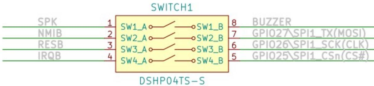
By default Neo6502 is shipped with all sections connected on the switch i.e. buzzer is enabled and all signals are wired to RP2040. This means you can't use SPI on UEXT connector if you do not disconnect these signals.
