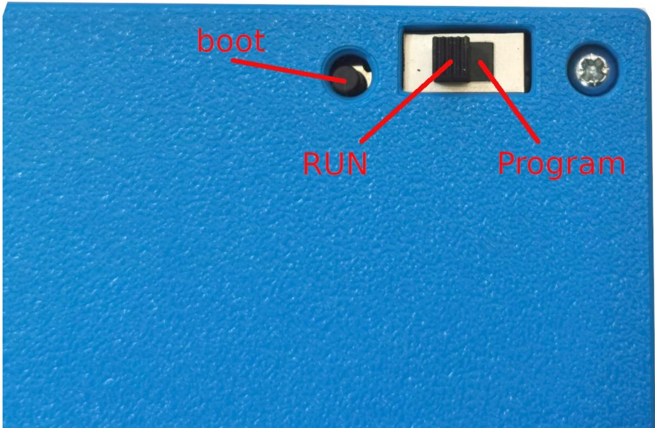
Switch the power ON and depress the boot button, you will see on your computer RP2 disk drive, drag and drop or copy the .uf2 file to this drive.
