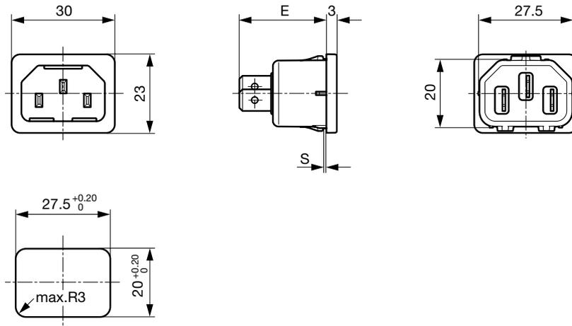
E: Lötanschlüsse 22.5 mm
