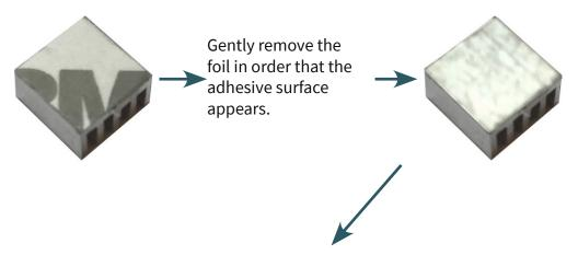
Now press the heat sink with light pressure on the chip so that the adhesive surface is pointing to the board.
