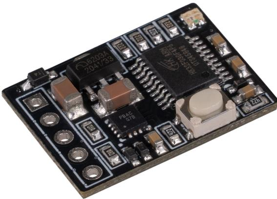
With this small module, you can trigger USB PowerDelivery protocols and thus, for example, charge your laptop via a PD-capable USB-C power supply unit. The output voltage can be adjusted in 5 steps (5 V, 9 V, 12 V, 15 V and 20 V) via the button integrated on the module as well as via the trigger input. The currently selected voltage can be read from the colour of the RGB LED integrated on the module. Due to its interfaces and design, the module can be used flexibly and is highly integrable.
