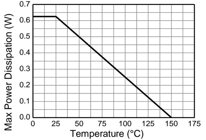
**Figure 2. Derating Curve**
