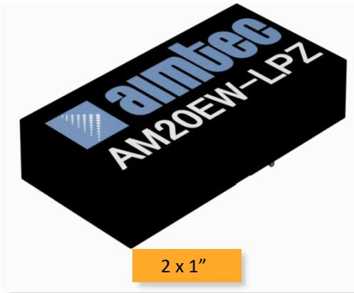
The AM20EW-LPZ is a 20W DC/DC converter that offers a regulated output which contributes to a more stable and reliable output performance. It features a wide 4:1 input voltage range of 9-160VDC, which will benefit your new system design.
