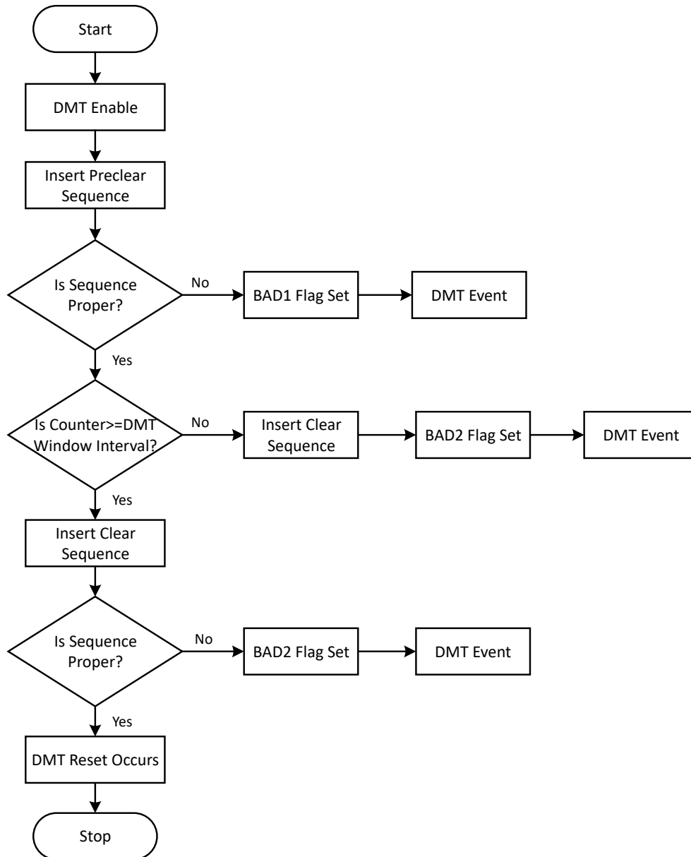
Figure 17-2. Flowchart for Clearing the DMT
