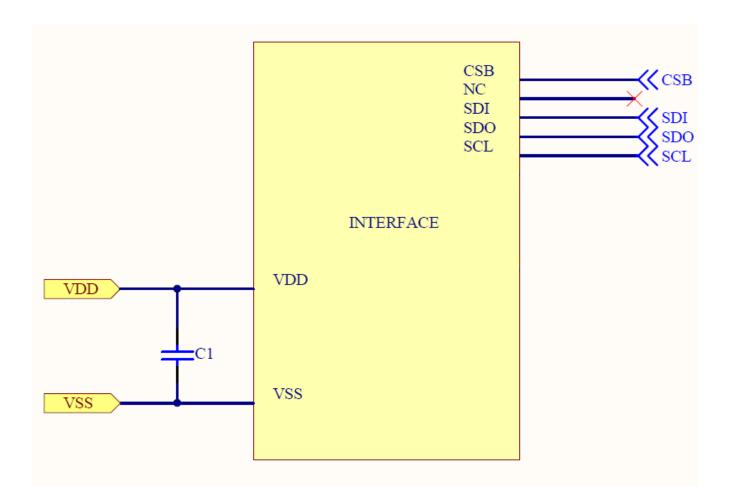
Pin connected to MCU interface: CSB,SDI,SDO,SCL
