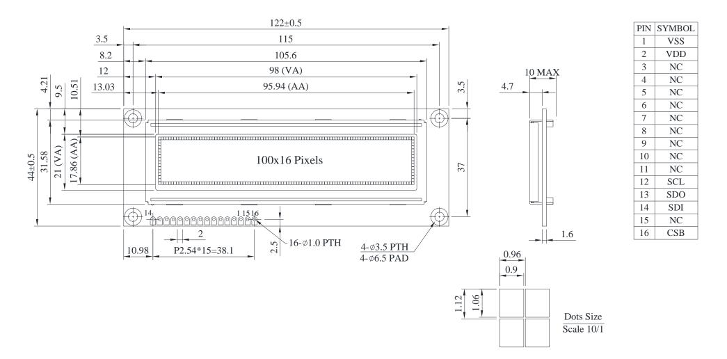
The non-specified tolerance of dimension is  $\pm 0.3 \text{ mm}$  .
