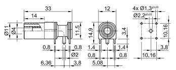
For mounting on printed circuit boards, touch-protected according to IEC/EN 61010-1. The socket is directly soldered onto printed circuit boards. The right-angled configuration minimizes the force transmitted to the printed circuit board through the plugged-in test lead. Right-angled  $\emptyset$  4 mm rigid socket accepting spring-loaded  $\emptyset$  4 mm plugs with rigid insulating sleeve.
