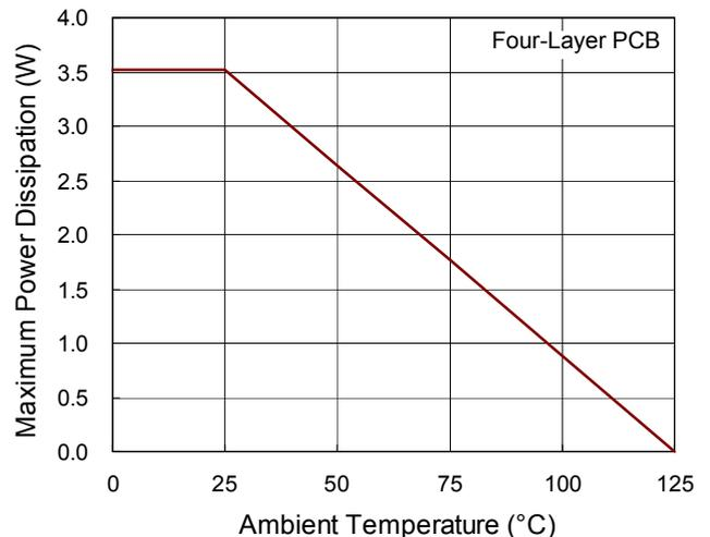
Figure 9. Derating Curve of Maximum Power Dissipation
