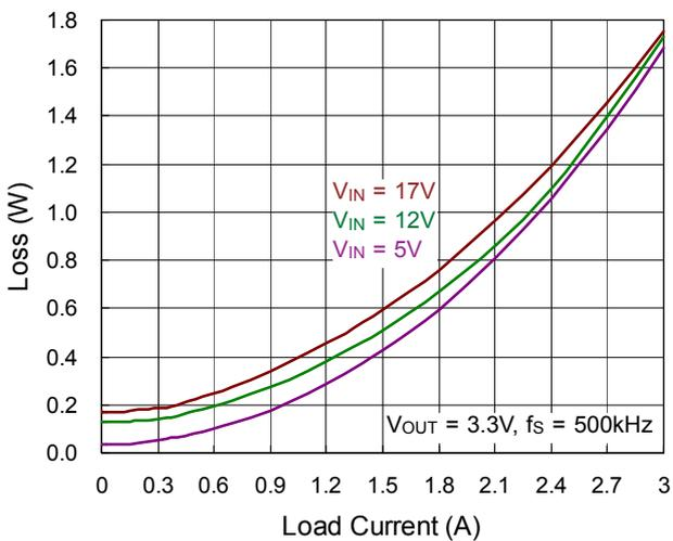
Figure 8. Channel 3 Loss vs. Load Current
