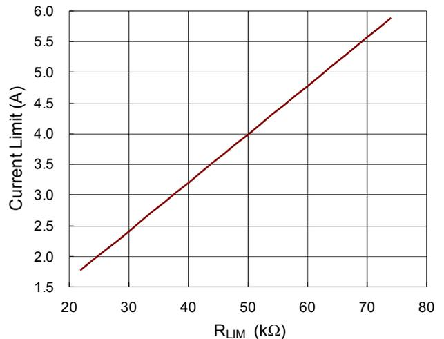
Figure 4. Channel 1 Current Limit vs. RLIM
