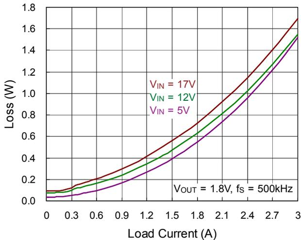
Figure 7. Channel 2 Loss vs. Load Current
