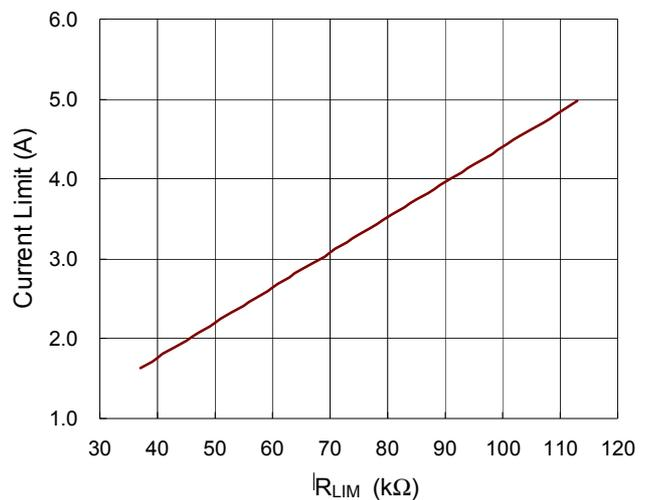
Figure 5. Channel 2 and Channel 3 Current Limit vs. RLIM
