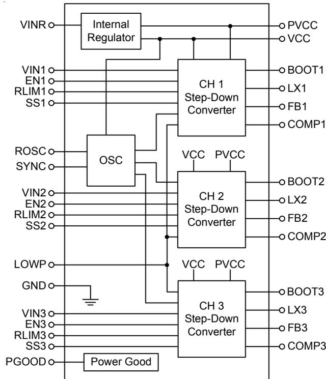
Each Channel Function Block Diagram
