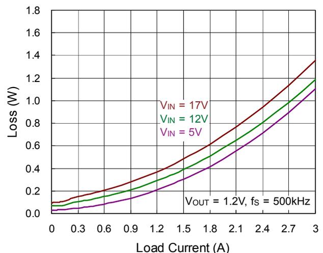
Figure 6. Channel 1 Loss vs. Load Current
