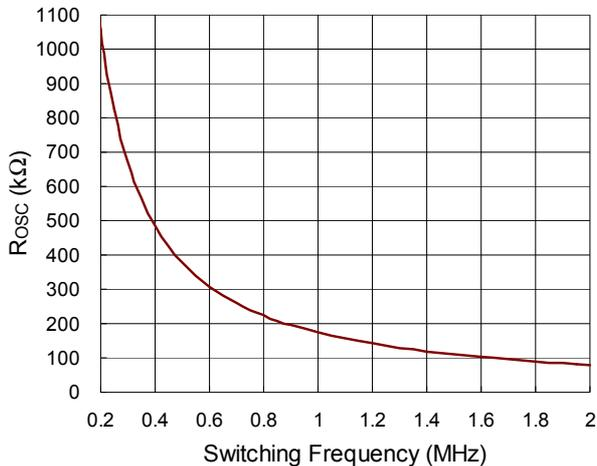
Figure 1. R<sub>OSC</sub> vs. Switching Frequency
