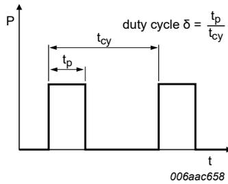
Fig. 13. Duty cycle definition
