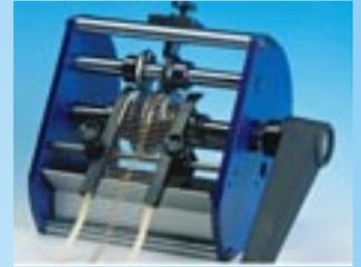
The TP6/V/21-EC machine is designed for cutting and bending taped axial components for vertical mounting. It operates components with lead diameters from 0,8 to 1,3 MM (.031 to .051"). The bending pitch is determined by the bending cam supplied and it can be changed by replacing this cam with one having different thickness.
