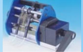
Machine model TP6/V-PR/2 is designed for cutting, bending and forming taped axial components for vertical mounting. The standard form locks the components into the P.C.Board. All dimensions are adjustable. This model handles components with lead diameters from 0,5 to 0,8mm (.019 to .031"). Special versions can be manufactured to form leads having different dimensions.
