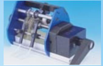
Machine model TP6/V-PR is designed for cutting, bending and forming taped axial components for vertical mounting. The standard form locks the components into the P.C.Board. All dimensions are adjustable. This model handles components with lead diameters from 0,5 to 0,8mm (.019 to .031"). Special versions can be manufactured to form leads having different dimensions. It is possible to suppress the form and only operate the "V" bend of components.
