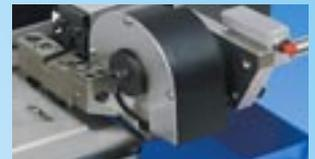
SEP 4 – STRIP CUTTING MACHINE. Quick and easy set up for various sizes, turning adjustment knob for header length of 1 to 32 pins. Hold down clamp for exact and sure positioning. DC motor with speed adjustment for optimal efficiency. Counter for keeping trace of the number of component cut.
