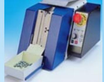
The TP/TC4 machine is designed to cut loose radial components. The speed and cutting length are adjustable. The machine stops when the front cover is removed. The length of the leads in origin must be  $L + 6$  mm minimum.
