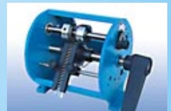
The model TP/FAST is designed to separate the connectors from the metal hinge keeping them properly gathered
