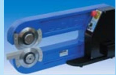
Motorized machine suitable to separate pre-assembled Electronic Board. Precise, reliable and safe. The PCB is manually fed between the lower and upper blades using the scoring as reference. By pushing the board horizontally, the blade rotation starts offering a sharp and accurate cut. The blade height is adjustable depending on the thickness of the PCB. Upper circular blade and lower linear blade are also available titanium plated
