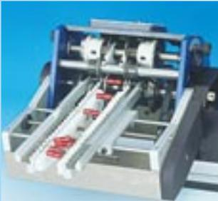
CS40 - 51.0400 FEEDER FOR LOOSE COMPONENTS
