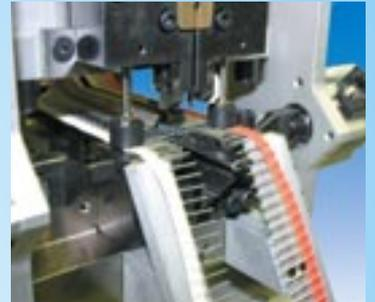
Olamef's knowledge and experience manufacturing forming machines are applied when designing this new line of equipment. It helps to eliminate manually forming and inserting through hole components.
