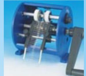
The TP6/S machine is designed for cutting and bending axial components for surface mount. The standard version offers the most common dimensions. Special versions to customer's specifications are available upon request. It is however necessary to know all dimensions of the component, before and after the bending operation.
