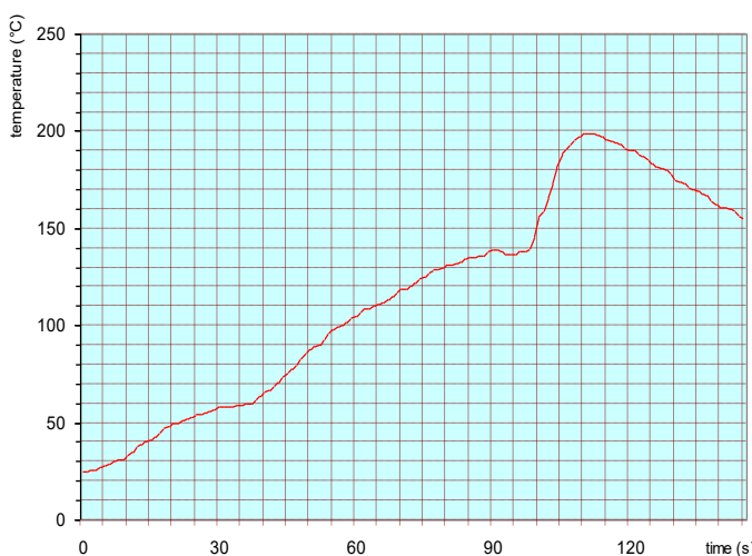
Example of a measured preheating profile
