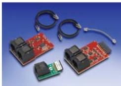
The optional Performance Pak consists of two circuit boards (driver and receiver) that employ two CAT5 cables. Debug pins are driven using LVDS communications, and additional trace connections allow high-speed serial trace uploads to the PC.
