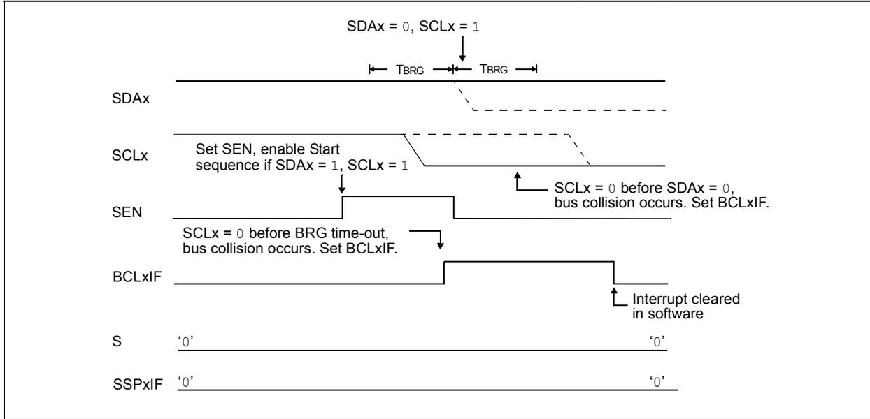
**FIGURE 19-30: BRG RESET DUE TO SDAx ARBITRATION DURING START CONDITION**
