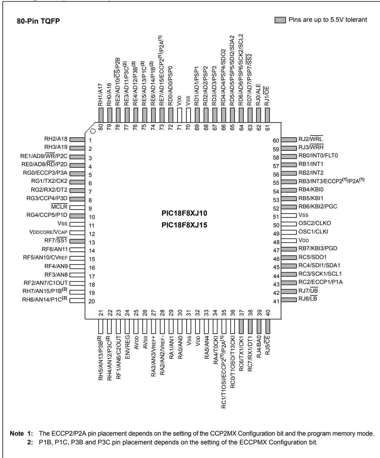
**Note 1:** The ECCP2/P2A pin placement depends on the setting of the CCP2MX Configuration bit and the program memory mode.
