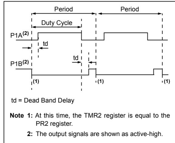
**FIGURE 18-5: EXAMPLES OF HALF-BRIDGE OUTPUT MODE APPLICATIONS**
