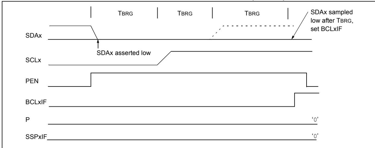
**FIGURE 19-34: BUS COLLISION DURING A STOP CONDITION (CASE 2)**
