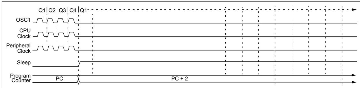
**FIGURE 4-6: TRANSITION TIMING FOR WAKE FROM SLEEP (HSPLL)**
