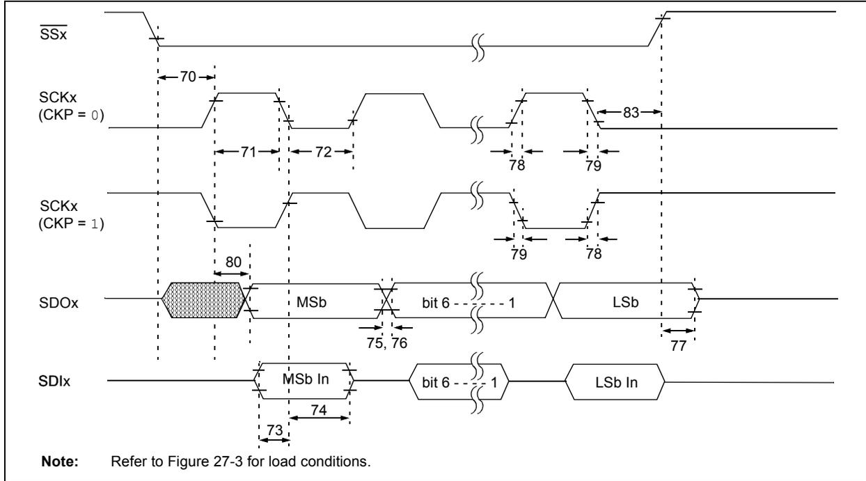
**TABLE 27-18: EXAMPLE SPI MODE REQUIREMENTS (SLAVE MODE TIMING, CKE = 0)**
