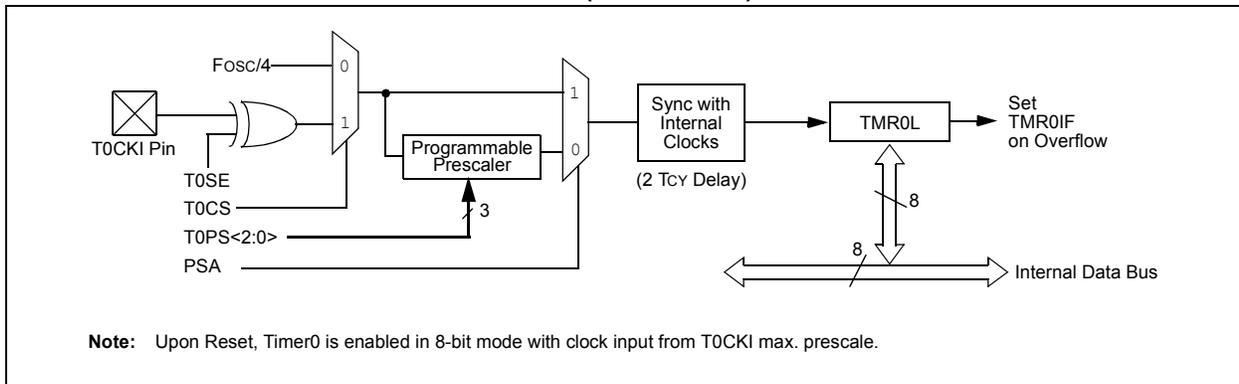
**FIGURE 12-2: TIMER0 BLOCK DIAGRAM (16-BIT MODE)**
