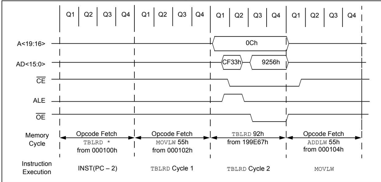
**FIGURE 8-5: EXTERNAL MEMORY BUS TIMING FOR SLEEP (EXTENDED MICROCONTROLLER MODE)**
