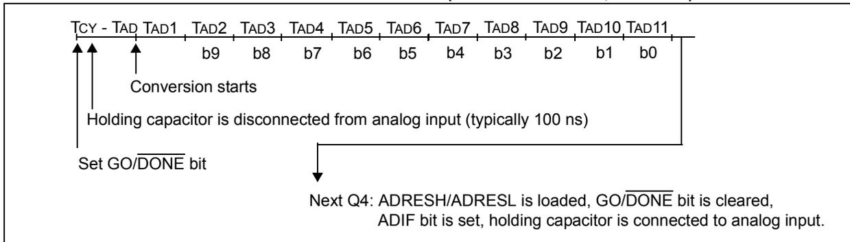
**FIGURE 21-4: A/D CONVERSION TAD CYCLES ( $\text{ACQT}\langle 2:0 \rangle = 010, \text{TACQ} = 4 \text{TAD}$ )**
