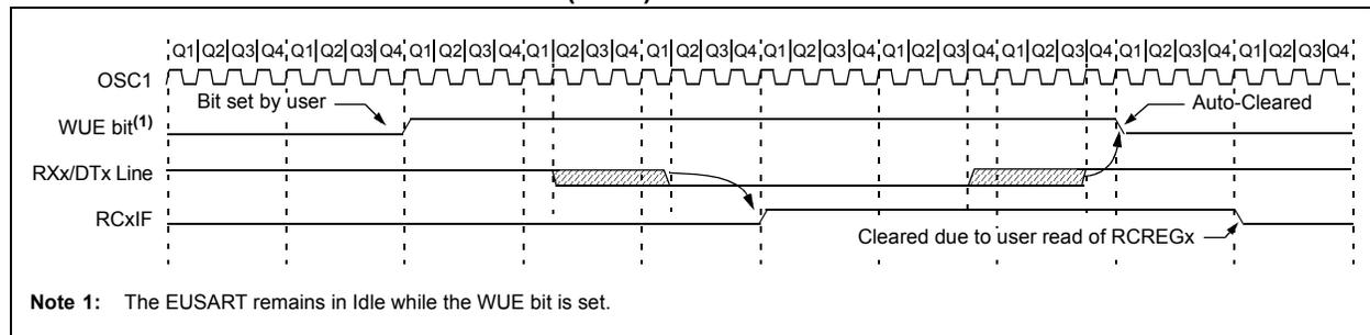
**FIGURE 20-9: AUTO-WAKE-UP BIT (WUE) TIMINGS DURING SLEEP**
