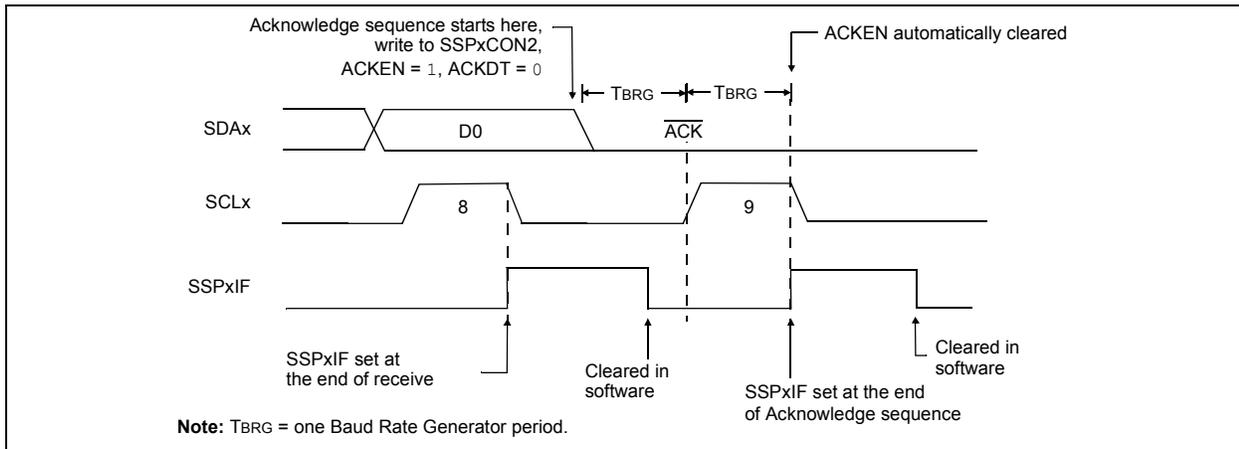
**FIGURE 19-26: STOP CONDITION RECEIVE OR TRANSMIT MODE**
