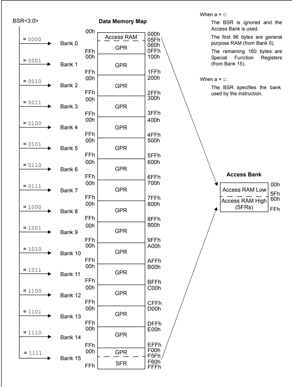
**FIGURE 6-9: USE OF THE BANK SELECT REGISTER (DIRECT ADDRESSING)**
