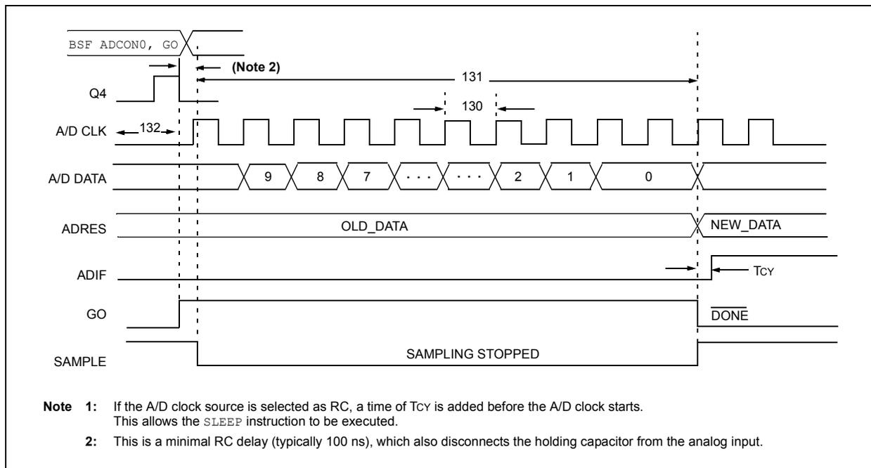
**Note 1:** If the A/D clock source is selected as RC, a time of  $T_{CY}$  is added before the A/D clock starts. This allows the **SLEEP** instruction to be executed.
