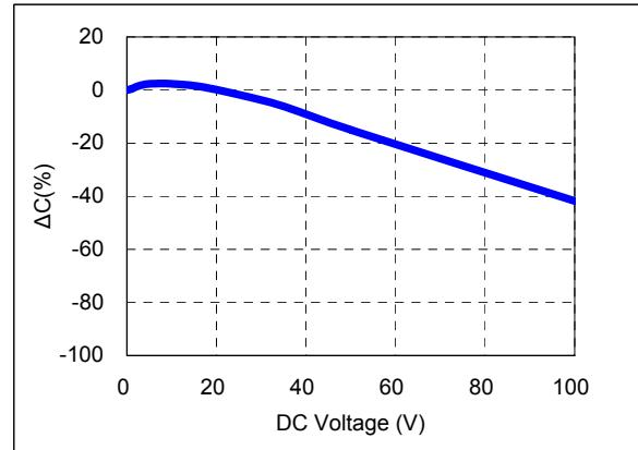
4) Bias TCC characteristics (Agilent 4284A, 1kHz, 1Vrms, 40Vdc)
