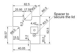
Enclosure with knob, for wall mounting, suitable for room thermostats etc. The knob fits among others potentiometer P/N. PCH215/30 from AB Electronik GmbH. Standard colour is white/white but other colours can be supplied upon request.
