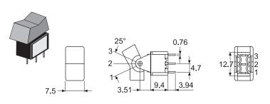
Rocker switch for 28V DC with white button. Available in 1 or 2 poles version and with 2 or 3 positions.
