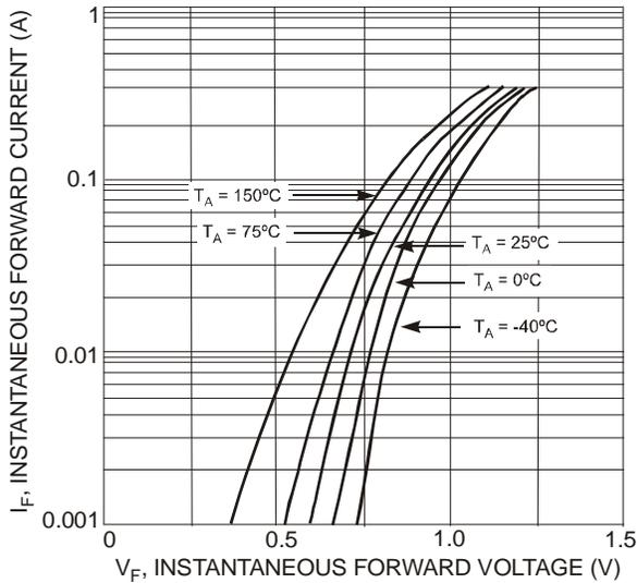
Fig. 1 Forward Characteristics
