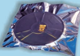
MBB with Recommended Light Air Evacuation
