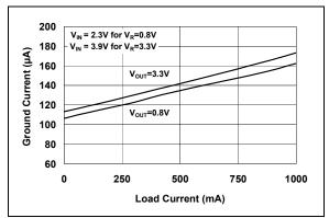
FIGURE 2-12: Ground Current vs. Load Current.
