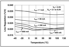
*FIGURE 2-16:* Line Regulation vs. Temperature.
