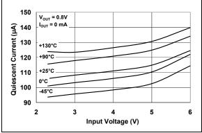
FIGURE 2-10: Quiescent Current vs. Input Voltage.
