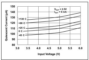
FIGURE 2-11: Quiescent Current vs. Input Voltage.
