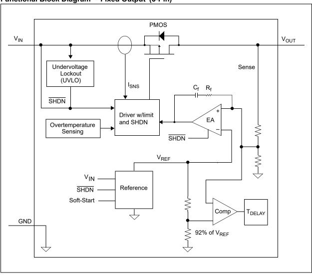
Functional Block Diagram – Fixed Output (3-Pin)
