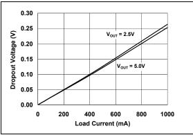
FIGURE 2-19: Dropout Voltage vs. Load Current.
