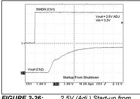
*FIGURE 2-26:* 2.5V (Adj.) Start-up from Shutdown.
