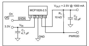
FIGURE 5-1: Typical Application Circuit.
