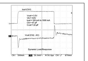
FIGURE 2-30: Dynamic Load Response (100 mA to 1000 mA).
