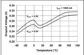
**FIGURE 2-20:** Dropout Voltage vs. Temperature.
