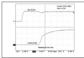
**FIGURE 2-25:** 2.5V (Adj.) Start-up from V<sub>IN</sub>.
