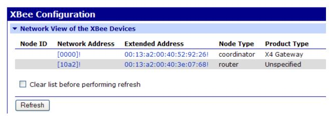
In the list under Network View of the XBee Devices, locate your product by its physical address. This address is printed on a label on the bottom of the unit. Click on the Network Address or Extended Address to open the product's settings page. 3. The XBee Network Configuration page is displayed.
