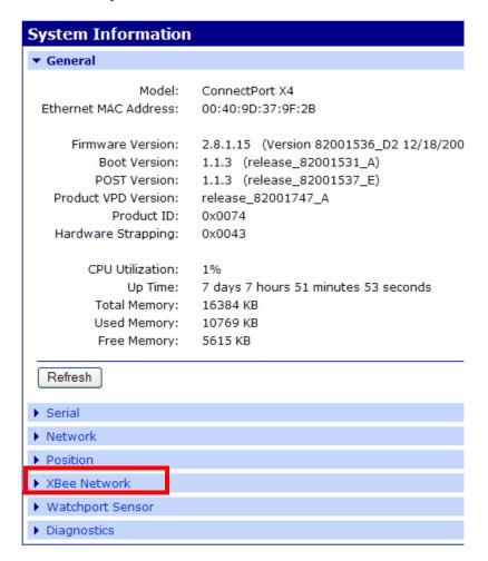
The **XBee Network** page is displayed. It shows several settings for the gateway, followed by the **Network View of the XBee Devices**.
