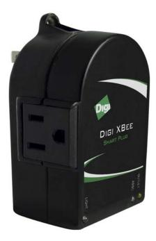
XBee technology enables low-cost, low-power networking of sensors, controllers and other devices in self-configuring, self-healing wireless networks. The XBee Smart Plug is an intelligent electrical outlet that can measure and control appliances plugged in via a standard electrical outlet. Part of Digi's Drop-in Networking family, XBee Smart Plug integrates with ConnectPort X gateways to centralize input from multiple XBee Smart Plugs into an energy management solution.
