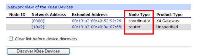
XBee 802.15.4 series products show the XBee module in the gateway as the **coordinator**, and any XBee Drop-in Networking Accessories as **end nodes**.
