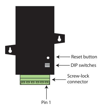
The adapter is switch-selectable between RS-422 half duplex/full duplex, and RS-485 modes (see "DIP switches" on page 25). The function for several pins varies between RS-422 and RS-485 modes.
