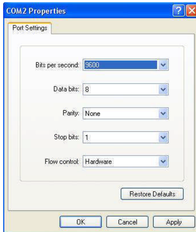
Figure 2-3 HyperTerminal Serial Settings
