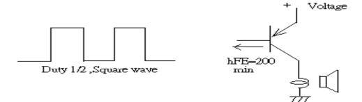
The base current Ib should high enough so that it saturates the collector current of the transistor with the CB load.
