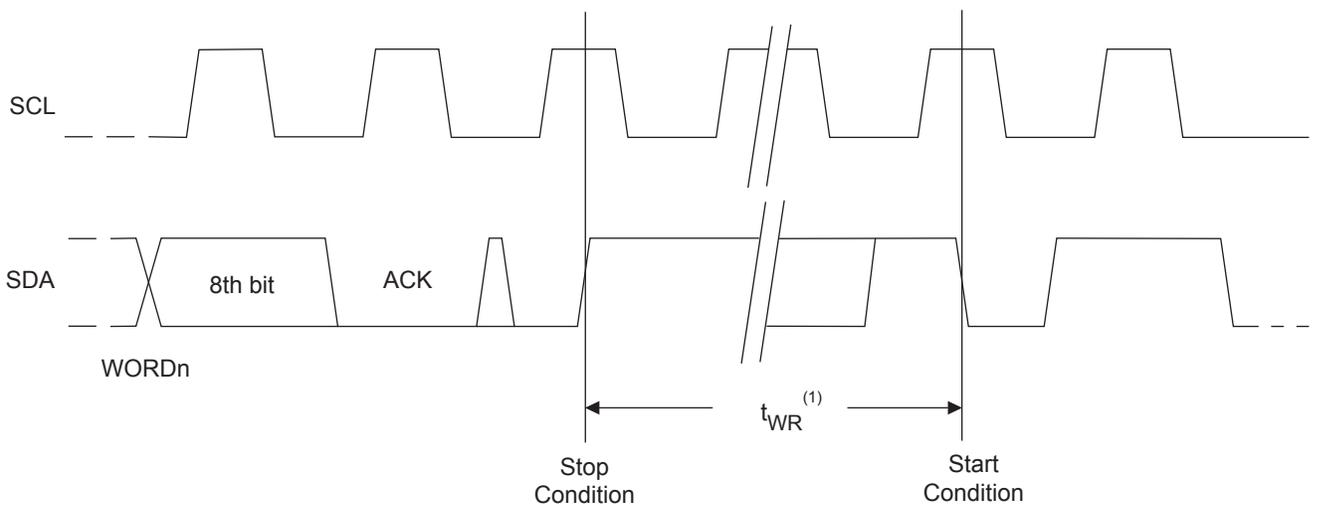
Notes: 1. The write cycle time  $t_{WR}$  is the time from a valid Stop condition of a write sequence to the end of the internal clear/write cycle.
