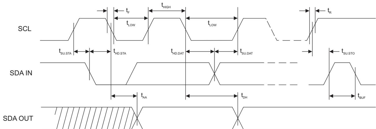
**Figure 5-3. Write Cycle Timing**
