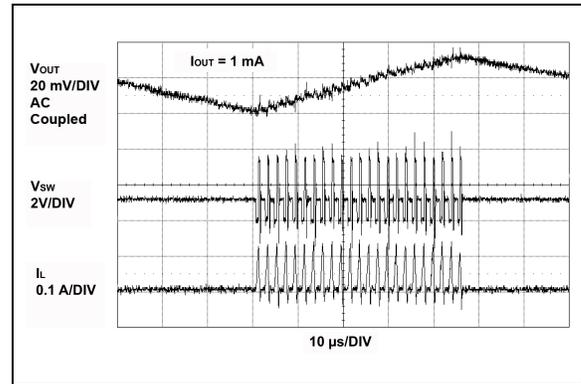
**FIGURE 2-16:** MCP1640 3.3V  $V_{OUT}$  PFM Mode Waveforms.
