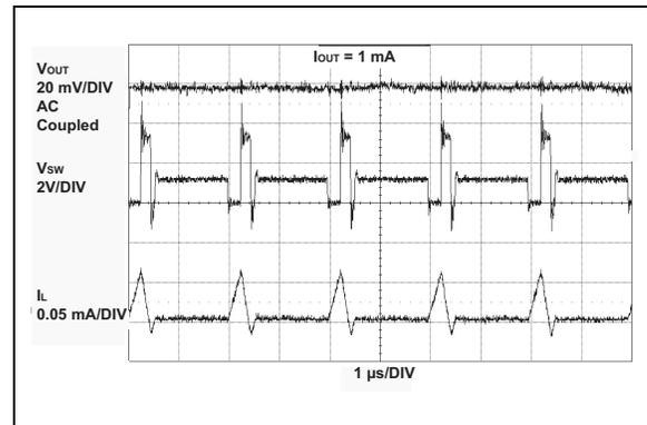
**FIGURE 2-17:** MCP1640B 3.3V  $V_{OUT}$  PWM Mode Waveforms.
