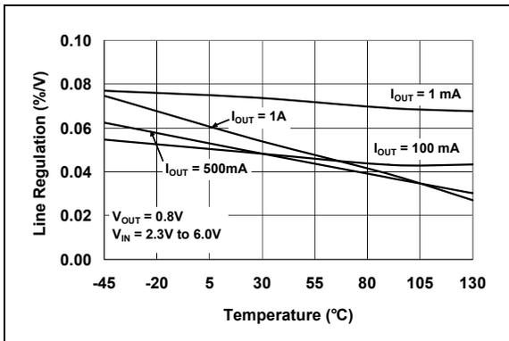
**FIGURE 2-15:** Line Regulation vs. Temperature (0.8V Fixed).
