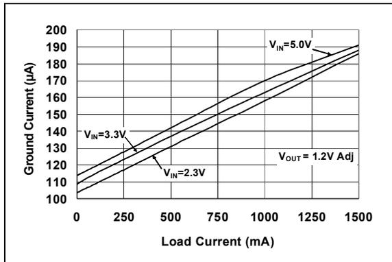
**FIGURE 2-2:** Ground Current vs. Load Current (1.2V Adjustable).
