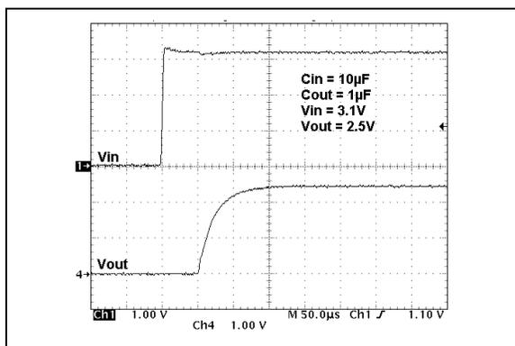
**FIGURE 2-27:** 2.5V (Adj.) Startup from  $V_{IN}$ .
