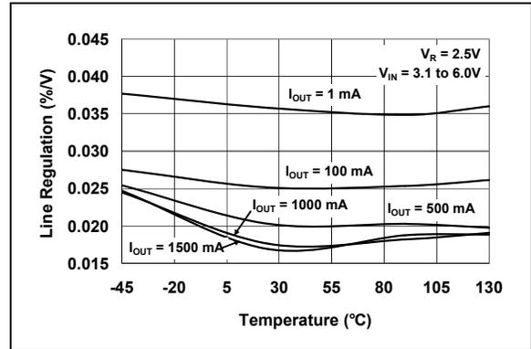
**FIGURE 2-16:** Line Regulation vs. Temperature (2.5V Fixed).
